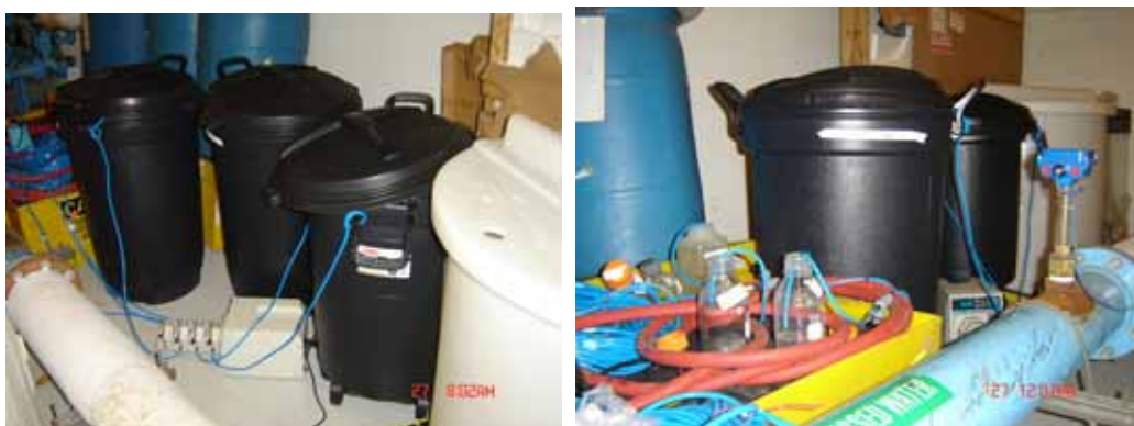
Figure 7.14. Sampling from the three pipe loop treatments. The reservoirs allowed free chlorinated or chloraminated water to be continuously pumped (using a peristaltic pump) through different sections of the pipe loop.
