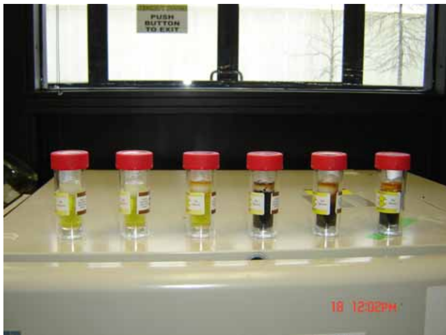
Figure 7.8. IRB-BART® system for iron-related bacteria.
