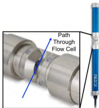
Figure 6.31. Online absorbance analyzer (Scanalyzer).
