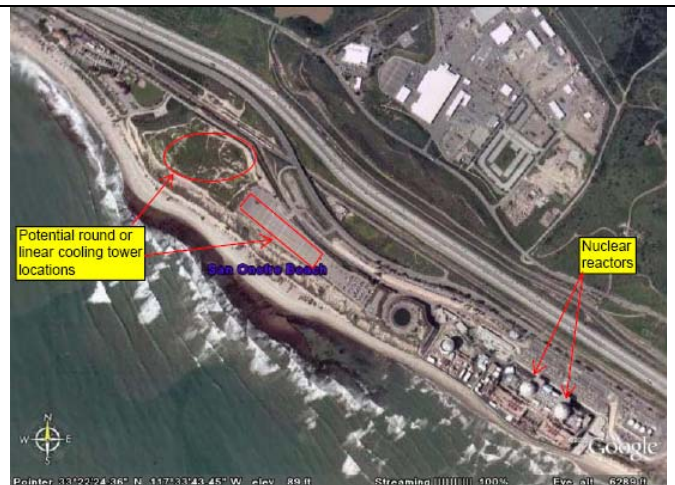
2,000 MW San Onofre - possible wet tower sites
