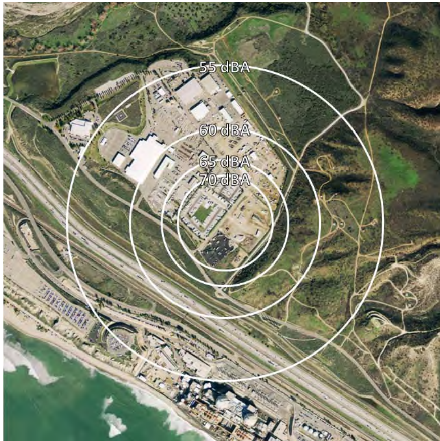
Figure 3.7 Noise impact of cooling towers without sound attenuation
