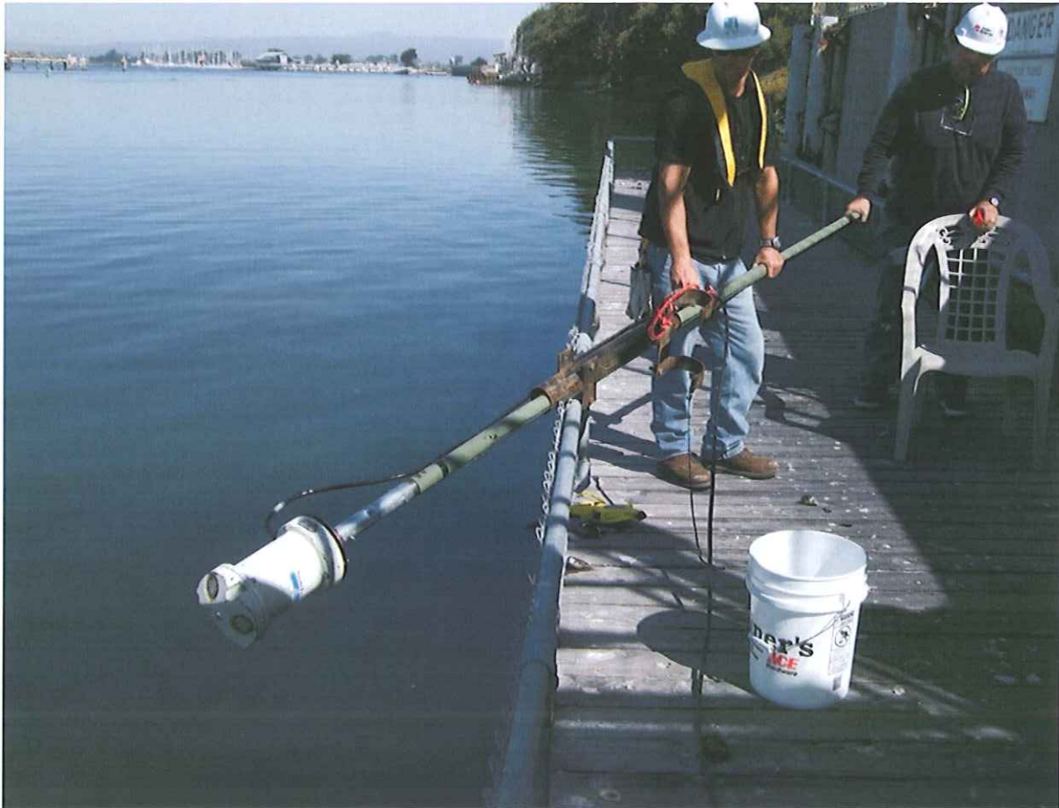
Figure 2-3. Sontek Acoustic Doppler Profiler (ADP) used for measuring intake approach velocities at the Moss Landing Power Plant Units 6 & 7 intake.
