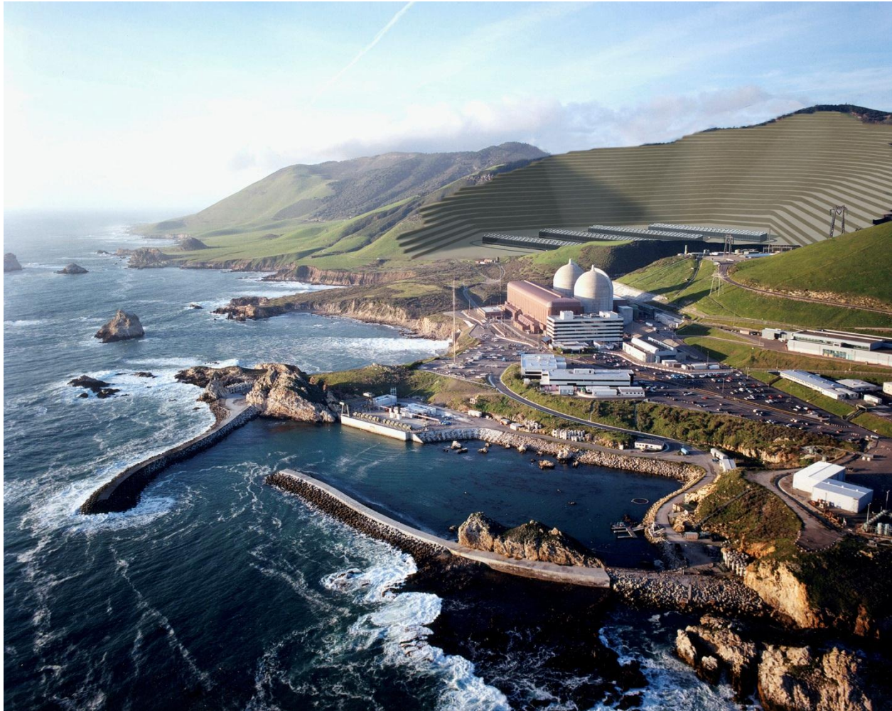
Figure 4.3-12. Mechanical (Forced) Draft Dry/Air-Cooling Site Configuration
