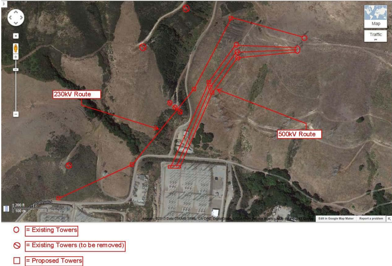
Figure 4.3-7. Existing 230 kV and 500 kV Power Line Rerouting
