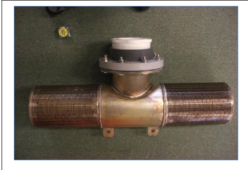
Figure 1. Wedgewire screen module used for Santa Cruz desalination plant pilot studies testing.
