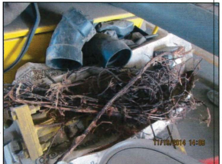
Photo 8: View of rooting bit with roots still attached to cutter
