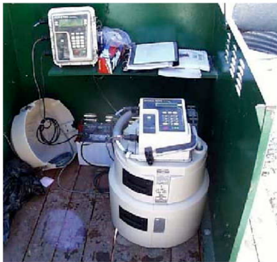
Figure 1-4 Typical monitoring equipment scenario at enclosed automated monitoring station. Shown are autosampler unit (lower right) and automatic flow meter (top left).
