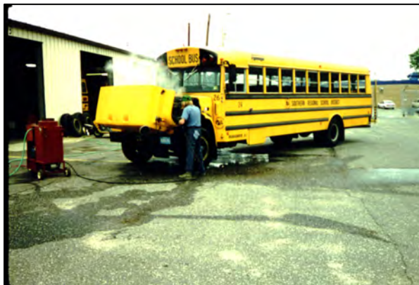
FIGURE 3-28 Washing of vehicle engine and allowing runoff to enter storm drainage system. SOURCE: Robert Pitt, University of Alabama.
