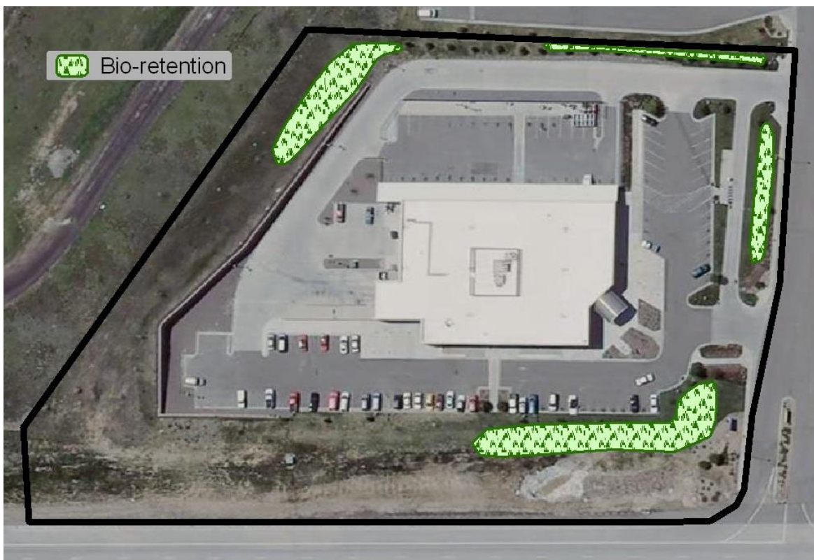
Figure 13. Actual Site and Onsite Control Measures (Denver, CO)
