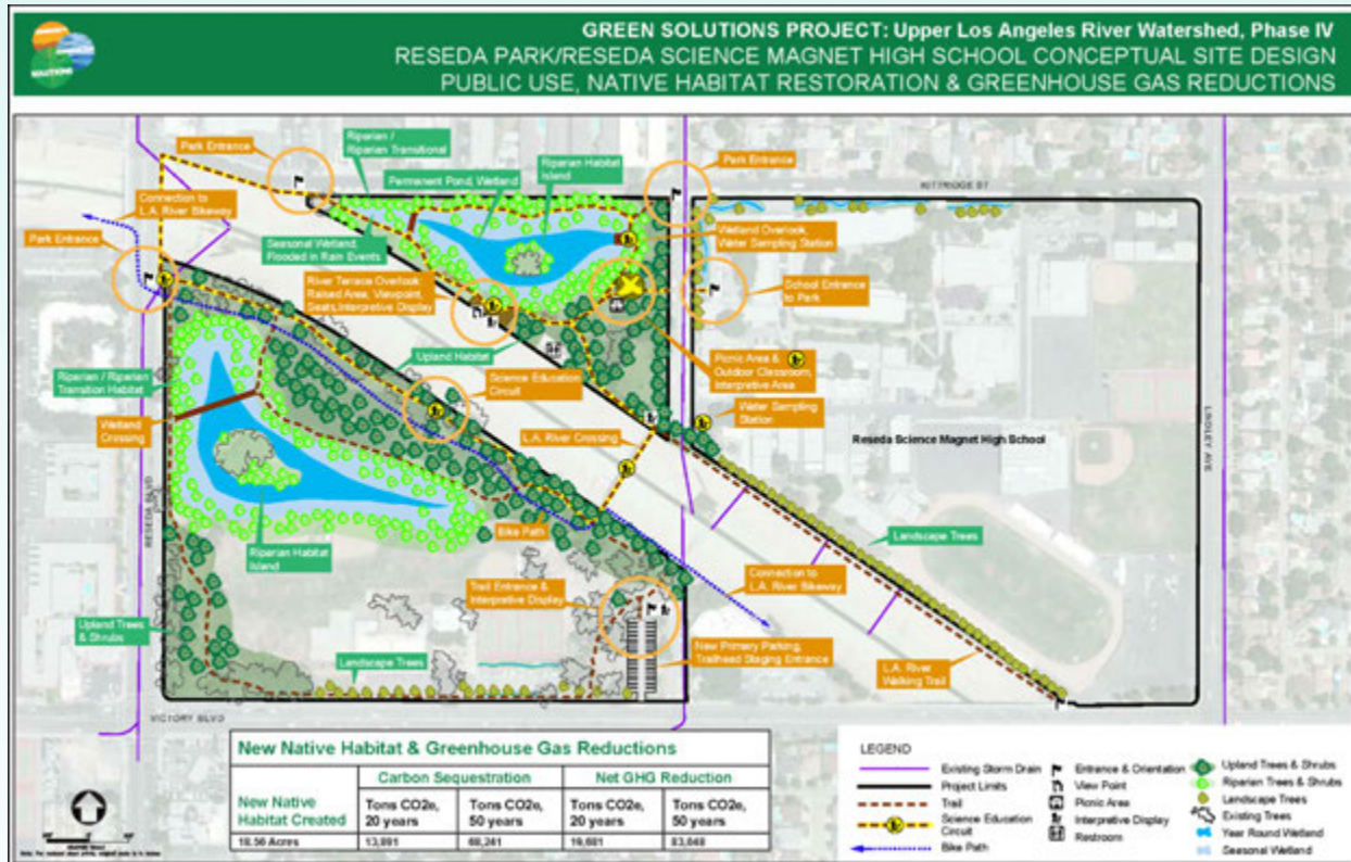
Figure VIII-3. Conceptual design for a regional project diverting runoff from a school site to offsite green infrastructure (Source: Community Conservation Solutions, 2016. Reprinted with Permission).
