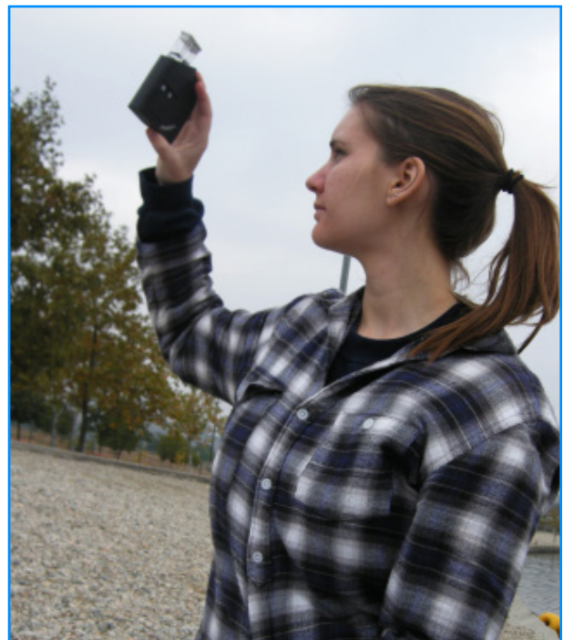
Jessie determines phosphate concentration using the Orbeco-Hellige color disc. Photos by Allison Sherris.
