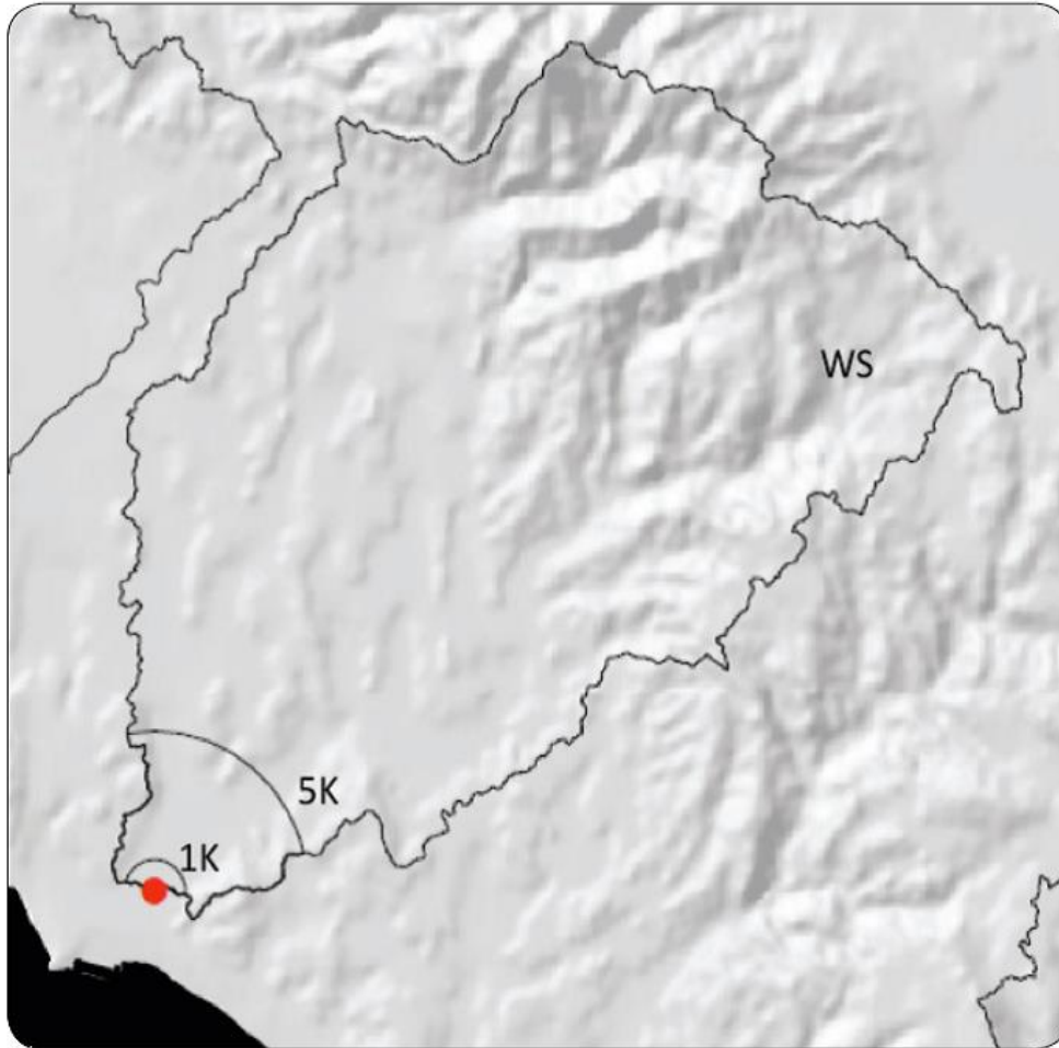
Figure 2. Drainage area delineation for watershed areas draining to SPoT sites. The larger polygon is the site's whole watershed (WS). The semi-circular smaller areas are watershed areas 1 km (1K) and 5 km (5K) upstream.
