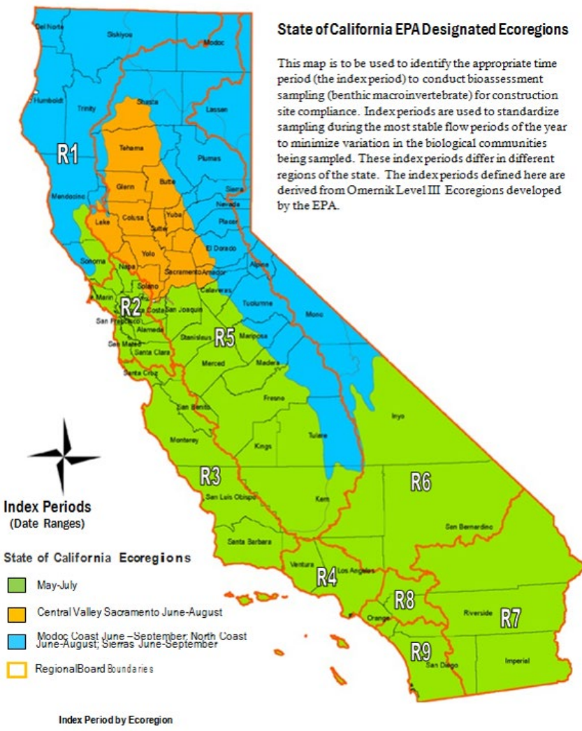
Figure 2. Index periods by ecoregion used as general guidelines for when to conduct bioassessment sampling. Local and/or annual weather conditions may be a sufficient reason to sample outside of the suggested date ranges (see text).
