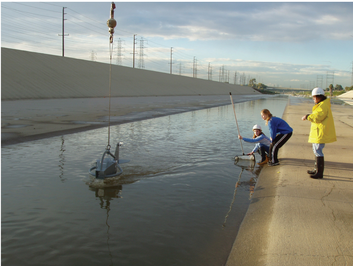
Figure 2. Concrete lined Coyote Creek, showing streambed sampler and hand net.
