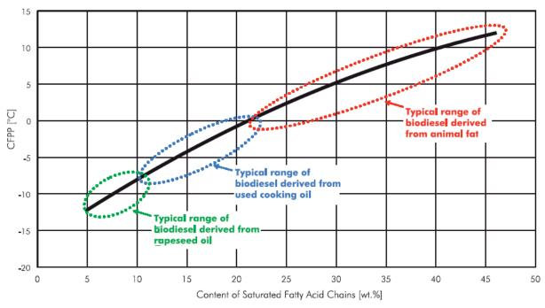
Figure 4.1. Relation between content of saturated fatty acids in biodiesel (without additives) and its CFPP value\*.
