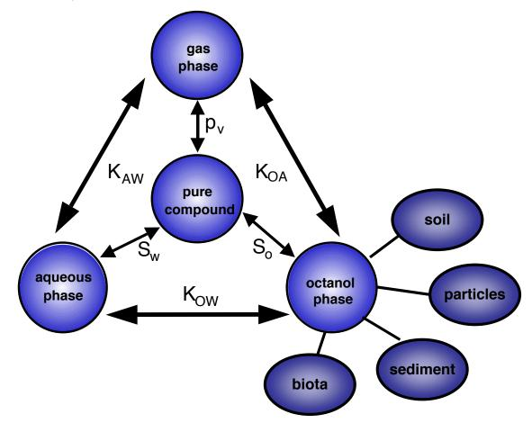
Figure 6.2. Phase distribution equilibria involving pure phase partition coefficients (water solubility S<sub>W</sub>, solubility in octanol S<sub>O</sub> and vapor pressure p<sub>V</sub>) showing the links for describing environmental phase partitioning (K<sub>AW</sub> air/water partition coefficient, K<sub>OW</sub> octanol/water partition coefficient, K<sub>OA</sub> octanol/air partition coefficient). The octanol phase is used for soil, sediment, particles and biota).
