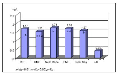
Figure 6.4. BOD<sub>5</sub> values for biodiesel and diesel\*.
