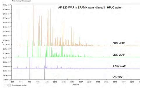
Figure II-B-4. Range finding experiment with increasing fractions of AF-B20 WAF\_01 in HPLC water. The optimal dilution for the SBSE analysis was identified as 25% WAF in HPLC water.
