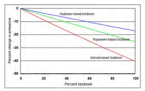
Figure 4.4. Biodiesel feedstock effect on CO emissions.
