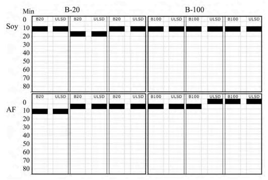
Figure II-C-4: Characteristic times to plume plume separation from the sand surface for each of the four blends (Soy B-20, Soy B-100, Animal Fat (AF) B-20, AF B-100) relative to ULSD in sideby-side comparison. The three columns per fuel blend show the results for each of the three replicates.
