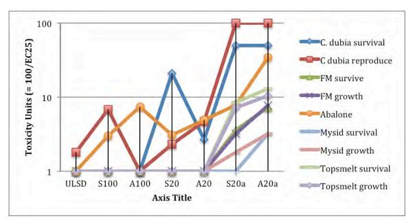
Figure 1. Toxicity scores (as Toxicity Units, =  $100/ \text{EC}_{25}$ ), for the different endpoints (e.g., survival, reproduction, growth) of 5 of the 6 species tested, as a function of fuel blend to which species was exposed. The graph is absent Green Algae that showed different behavior than the trend observed here.
