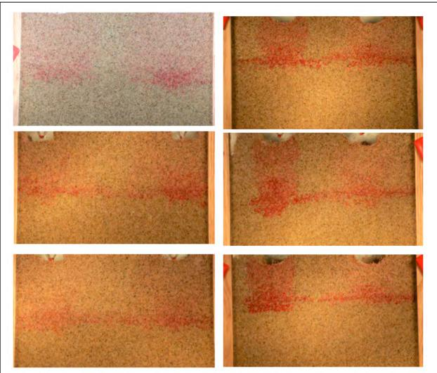
Figure II-C-2. Example final digital images. Left panel: the triplicate images for Soy B-20 at 2 hours; the left hand plume is Soy B-20 and the right-hand plume is ULSD. Right pane: those for the Animal Fat B-100 at 2 hours; the left hand plume is Animal Fat B-100 and the right-hand plume is ULSD. Note the greater color density indicating increased residual of the Animal Fat B-100 in the vadose zone and the thicker lens formation on the water table, with respect to that of ULSD.
