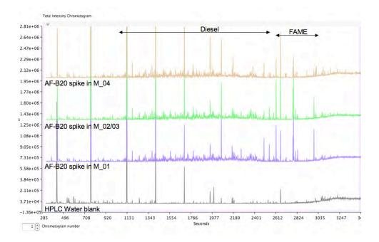
Figure II-B-3. Overlay of 1:1000 (v/v) dilution of neat AF-B20 fuel in MeOH spiked (4  $\mu$ L) in each of the test waters (40 mL). The HPLC water blank is 40 mL of the water used as makeup volume in the WAF analysis. The large evenly spaced peaks are siloxanes from the stir-bar coating and are not quantified in the method.
