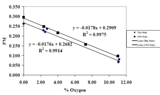
Figure 4.7. Regression model showing effect of oxygen on particulate matter\*.
