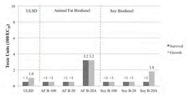
Effects on the mysid survival and growth endpoints were either absent or very low (< 1 or 1.0 TUc) for the USLD, and all biofuels and mixtures tested except those containing additive. The AF B-20A exhibited 3.2 TUc to both endpoints, while the Soy B-20A produced 1.8 TUc to the growth endpoint.
