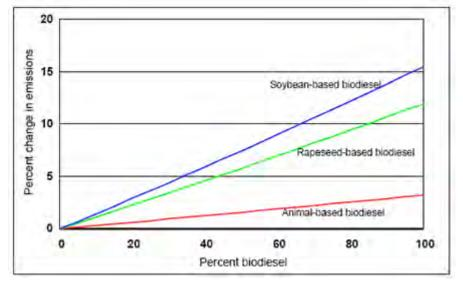
Figure 4.5. Biodiesel feedstock effect on NO<sub>x</sub> emissions\*.
