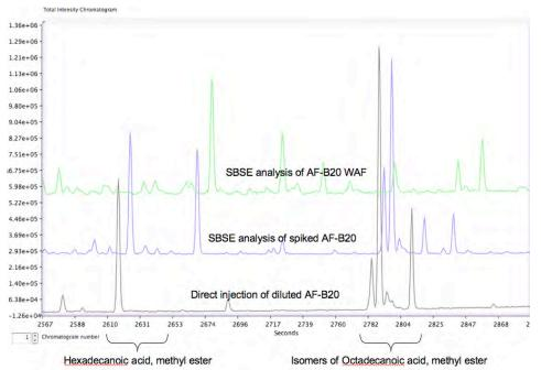
Figure II-B-5. Zoomed overlay in the region of the chromatogram where FAME elutes showing the presence of hexadecanoic acid methyl ester and the isomers of octadecanoic acid methyl ester in the raw fuel and in the spiked water but significantly reduced or absent in the WAF. The peak eluting at about 2660 seconds in the SBSE chromatograms is a siloxane from the stir bar and not part of the WAF or fuel.
