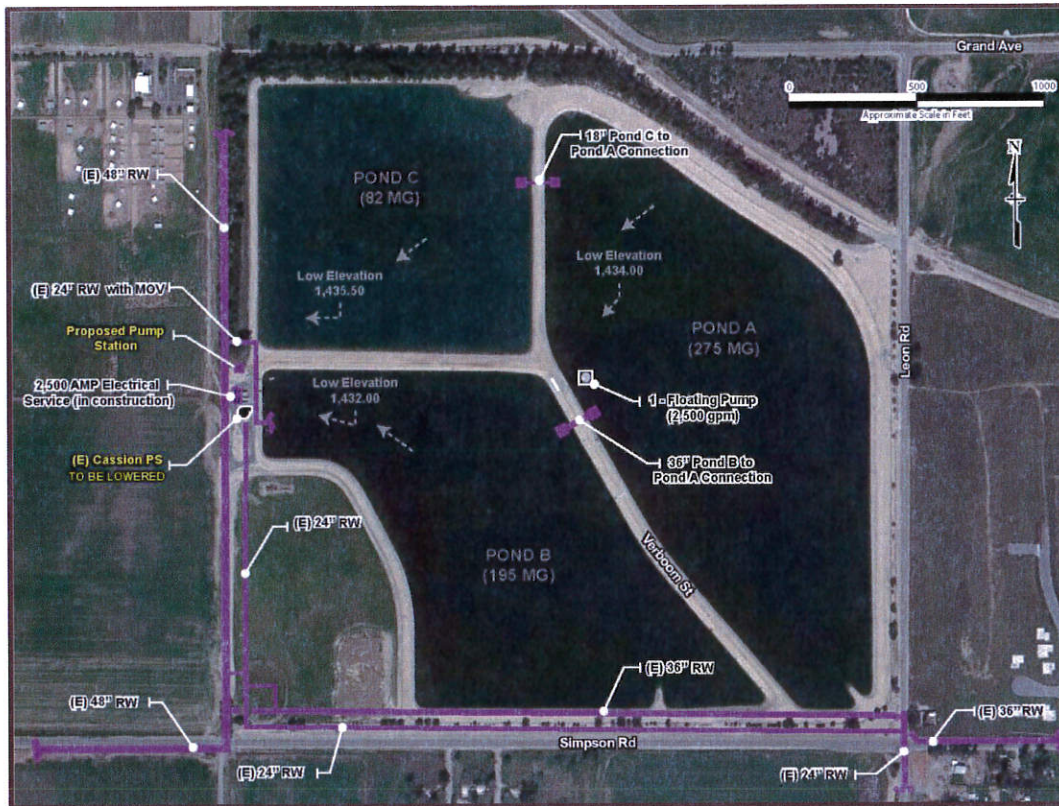
Figure 1-11 Winchester Recycled Water Storage Ponds Optimization Alternative 2
