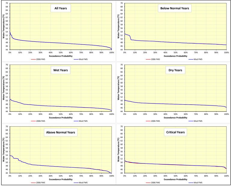
Figure F-2. Daily water temperature exceedance distributions during April below Keswick Dam on the Sacramento River over the 82-year simulation period.
