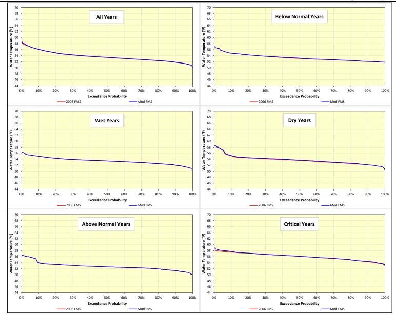
Figure F-12. Daily water temperature exceedance distributions during July at Balls Ferry on the Sacramento River over the 82-year simulation period.
