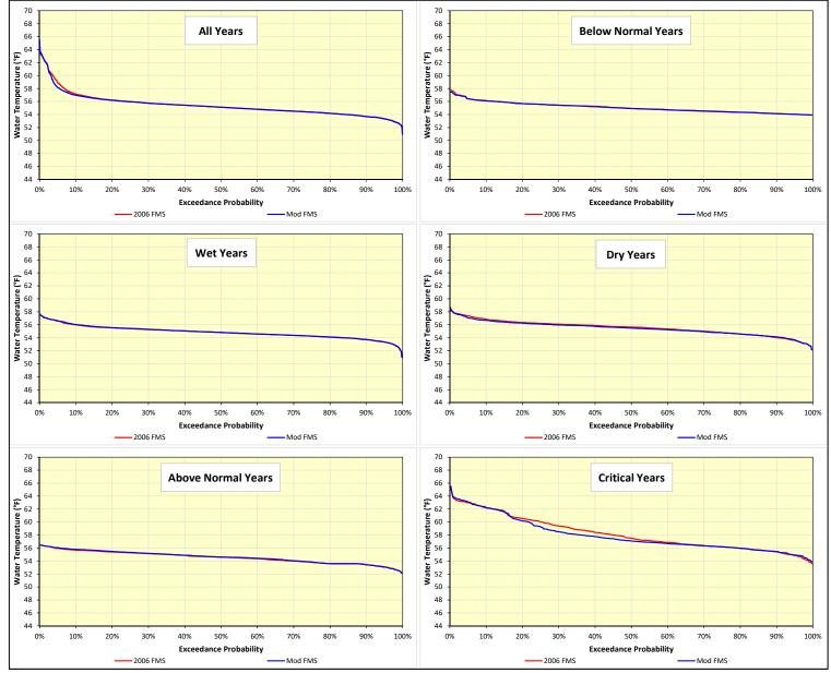
Figure F-15. Daily water temperature exceedance distributions during October at Balls Ferry on the Sacramento River over the 82-year simulation period.
