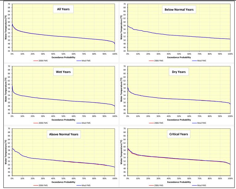
Figure F-10. Daily water temperature exceedance distributions during May at Balls Ferry on the Sacramento River over the 82-year simulation period.
