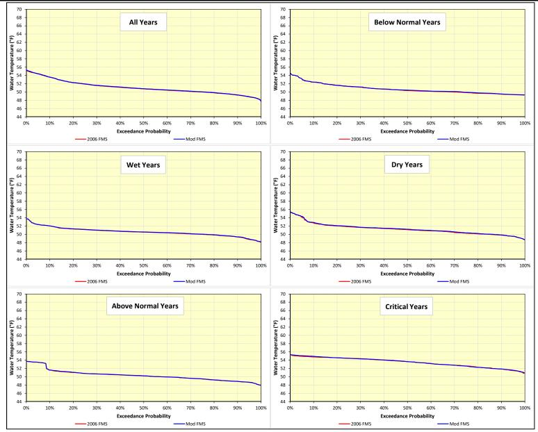
Figure F-5. Daily water temperature exceedance distributions during July below Keswick Dam on the Sacramento River over the 82-year simulation period.
