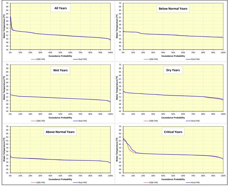
Figure F-6. Daily water temperature exceedance distributions during August below Keswick Dam on the Sacramento River over the 82-year simulation period.
