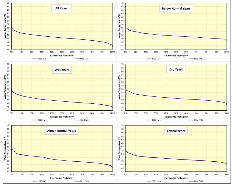
Figure F-9. Daily water temperature exceedance distributions during April at Balls Ferry on the Sacramento River over the 82-year simulation period.
