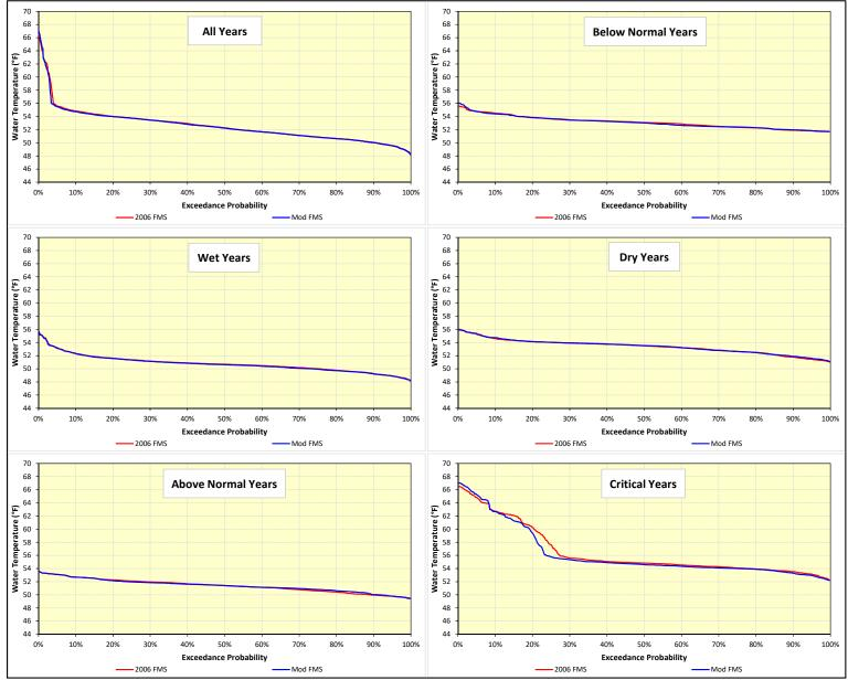
Figure F-7. Daily water temperature exceedance distributions during September below Keswick Dam on the Sacramento River over the 82-year simulation period.
