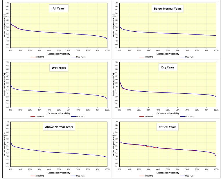
Figure F-11. Daily water temperature exceedance distributions during June at Balls Ferry on the Sacramento River over the 82-year simulation period.
