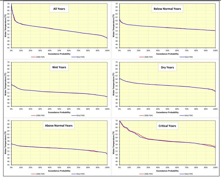
Figure F-14. Daily water temperature exceedance distributions during September at Balls Ferry on the Sacramento River over the 82-year simulation period.
