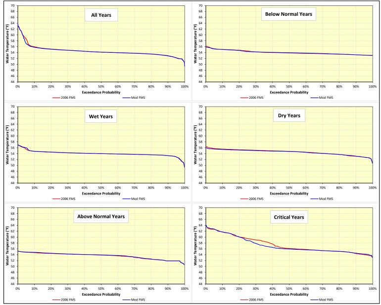
Figure F-8. Daily water temperature exceedance distributions during October below Keswick Dam on the Sacramento River over the 82-year simulation period.
