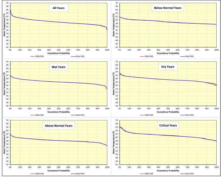
Figure F-20. Daily water temperature exceedance distributions during August at Red Bluff on the Sacramento River over the 82-year simulation period.
