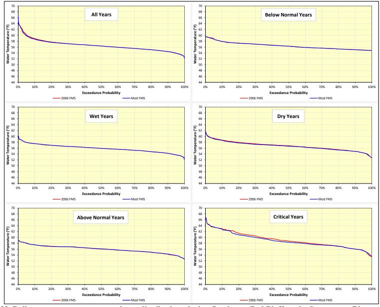
Figure F-22. Daily water temperature exceedance distributions during October at Red Bluff on the Sacramento River over the 82-year simulation period.
