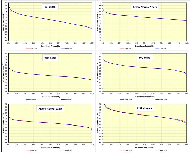
Figure F-21. Daily water temperature exceedance distributions during September at Red Bluff on the Sacramento River over the 82-year simulation period.
