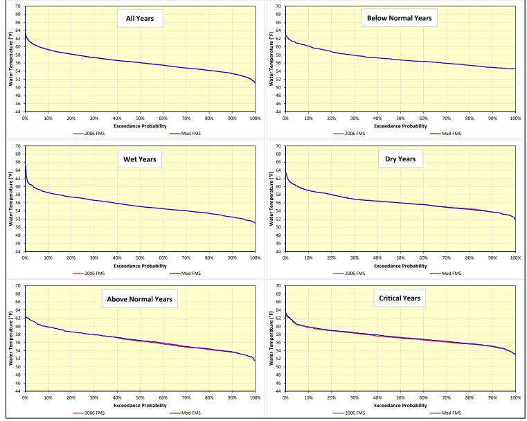
Figure F-17. Daily water temperature exceedance distributions during May at Red Bluff on the Sacramento River over the 82-year simulation period.
