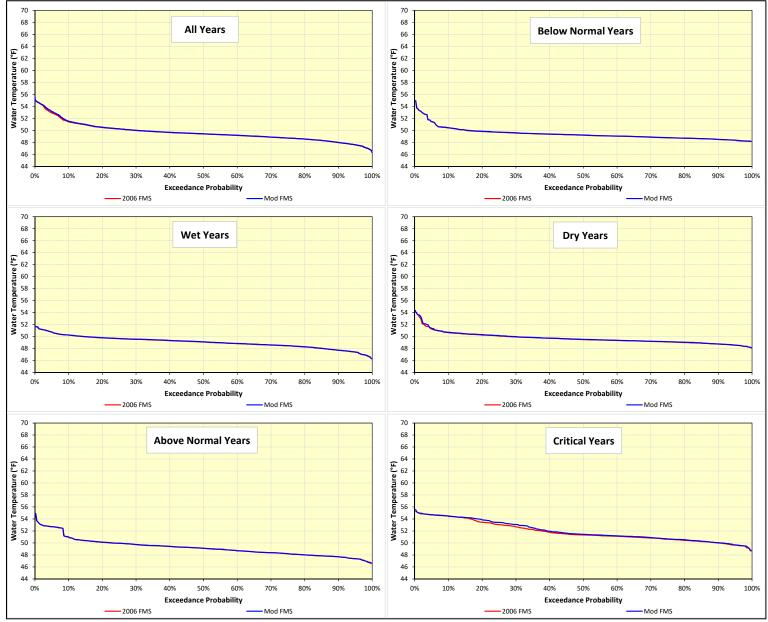
Figure F-4. Daily water temperature exceedance distributions during June below Keswick Dam on the Sacramento River over the 82-year simulation period.
