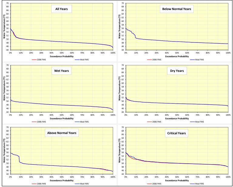
Figure F-3. Daily water temperature exceedance distributions during May below Keswick Dam on the Sacramento River over the 82-year simulation period.
