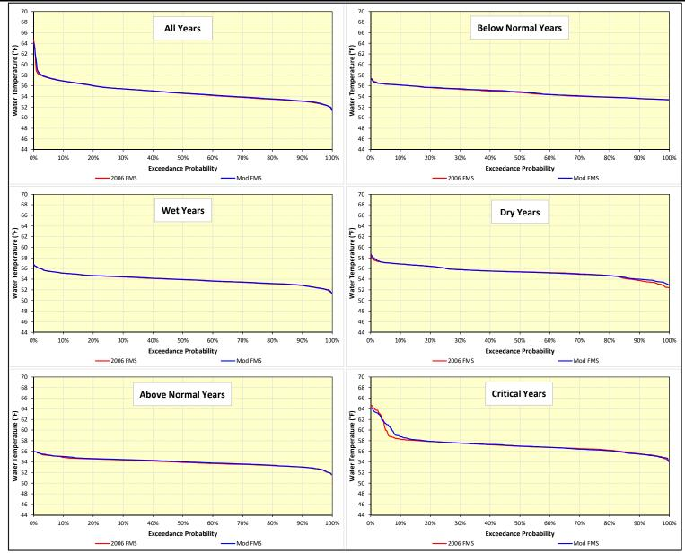
Figure F-13. Daily water temperature exceedance distributions during August at Balls Ferry on the Sacramento River over the 82-year simulation period.
