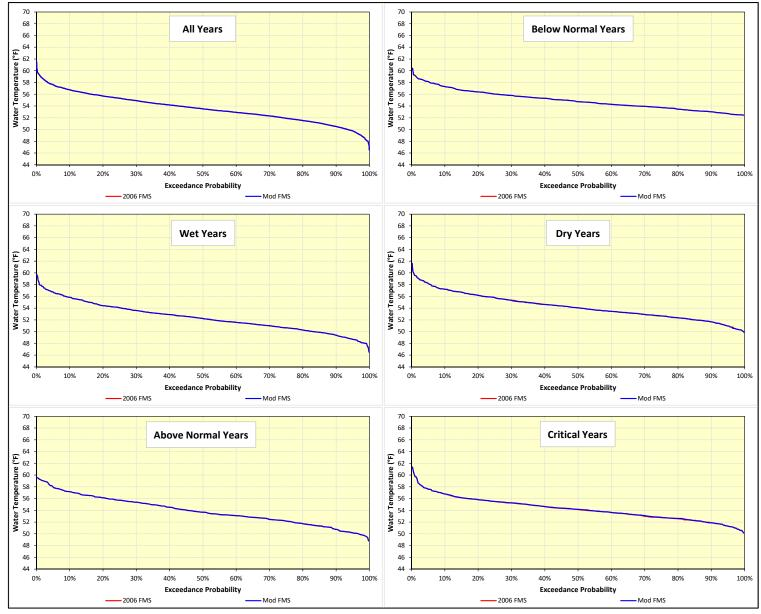
Figure F-16. Daily water temperature exceedance distributions during April at Red Bluff on the Sacramento River over the 82-year simulation period.
