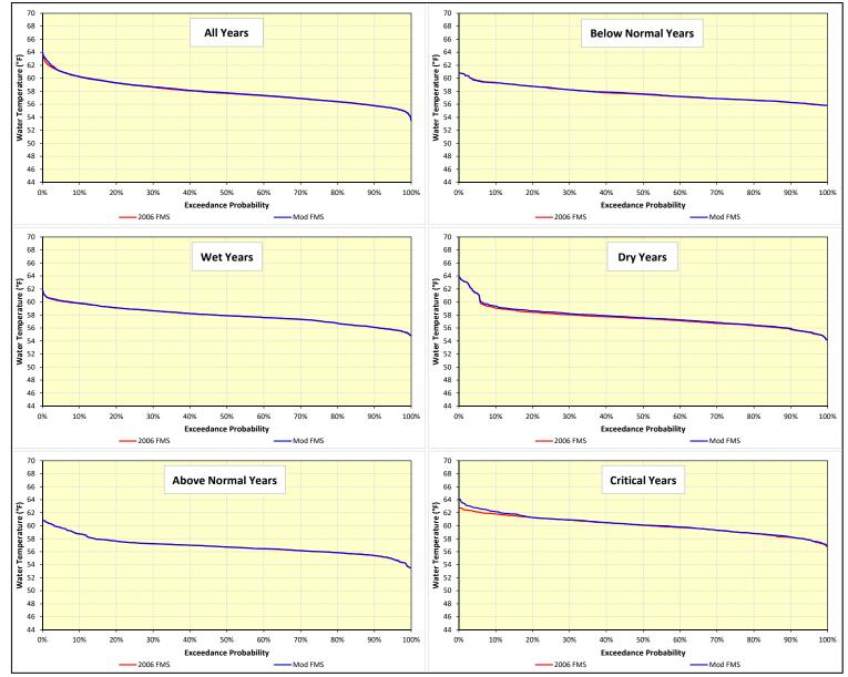
Figure F-19. Daily water temperature exceedance distributions during July at Red Bluff on the Sacramento River over the 82-year simulation period.
