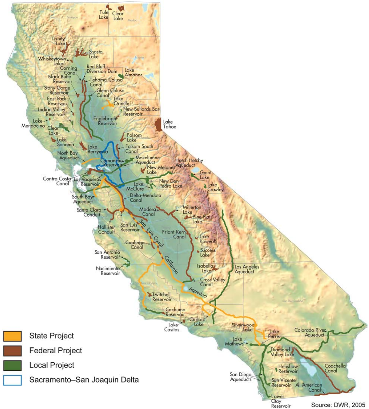
FIGURE 1-1 Major CVP and SWP Storage and Conveyance Facilities
