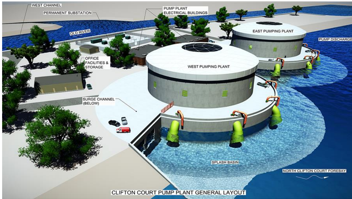
FIGURE 5: PROPOSED PUMPING FACILITIES AT CLIFTON COURT FOREBAY
