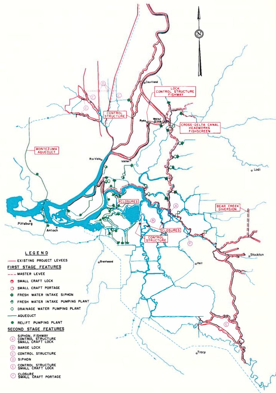
About 1,900 acres of Delta land would be filled with excess dredged material, and most of this land would be available for recreational development. The additional gates on the Cross-Delta Canal headworks and the extensions of the adjacent highway and railroad bridges would be constructed with about 16 feet of clearance above the present average water level to improve small craft access between the Sacramento River and channels of the Mokelumne River system.
