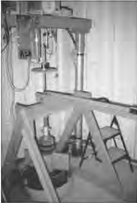
Figure 19 Photograph of extensometer
