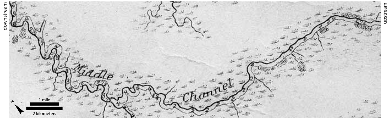
Figure 6.12. Channel depths on the Middle River decrease upstream. This 1850 map shows soundings in fathoms decreasing upstream (towards the right) from 3 to 9 fathoms (18-54 feet / 5.5-16.5 m) close to its mouth on the San Joaquin and about 2 fathoms (12 feet / 3.7 m) close to its head on Old River. The surveying was performed during periods of high flow in June. (Gibbes 1850a, courtesy of the Map Collection of the Library of UC Davis)
