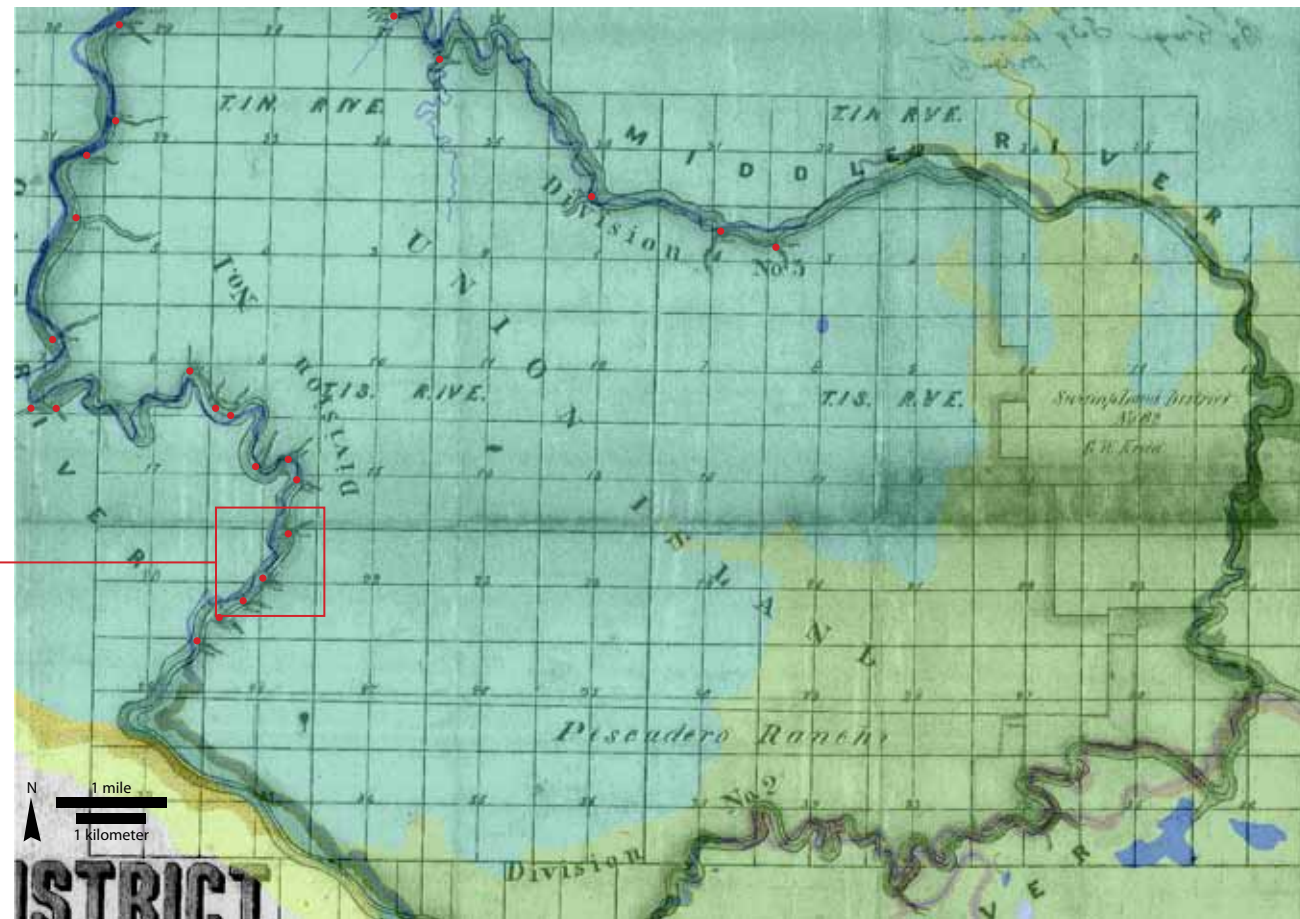
Figure 6.14. Channels large enough to dam become sparse where rivers are bordered by natural levees. These channels (red dots) are found only along lower (or the north part of) Union Island, as shown in this 1876 reclamation map. Natural levees became more substantial and limited the formation of these networks. Also, tidal energy was lower and therefore did not establish a dense network of channels. This transition is represented in the habitat type map with the appearance of willow riparian scrub along the mainstem channels and non-tidal wetland on the floodplain. These were significant tidal channels, as suggested by the dams that are indicated at the mouth of each channel, as shown below. (Wallace 1876, courtesy of the California State Lands Commission)
