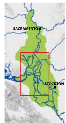
Figure 4.5. Comparing the planform of the San Joaquin distributaries to those of the Sacramento reveals the more deltaic pattern with sinuous branching channels associated with the San Joaquin, as shown in this State Engineering Department map. (Hall ca. 1880b, courtesy of the California State Archives)
