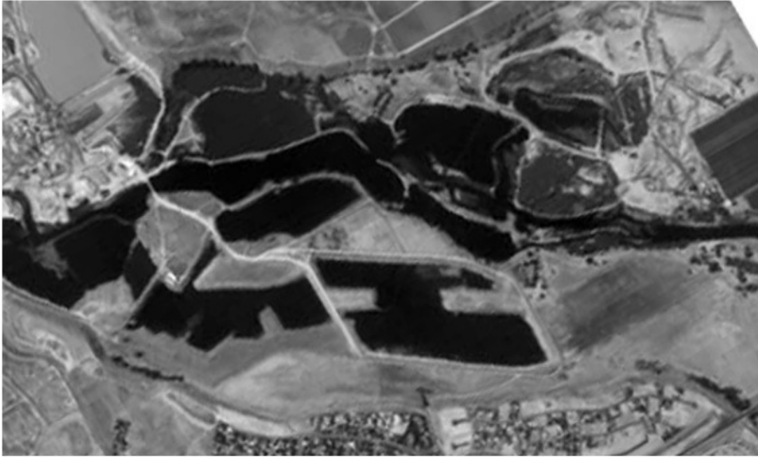
Instream and floodplain gravel mining pits at San Joaquin River at RM 254 in 1993. .
