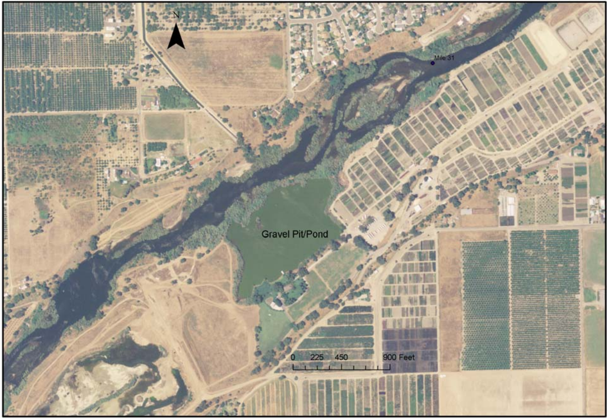
Figure 8. 4,030 – 4,070 cfs ponds visible and connected to channel RM 30.5.
