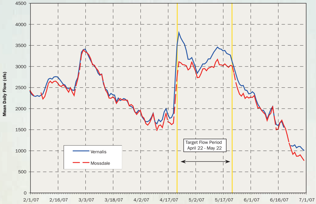
Figure 2-2 2007 VAMP - Flow Comparison, San Joaquin River near Vernalis and San Joaquin River at Mossdale
