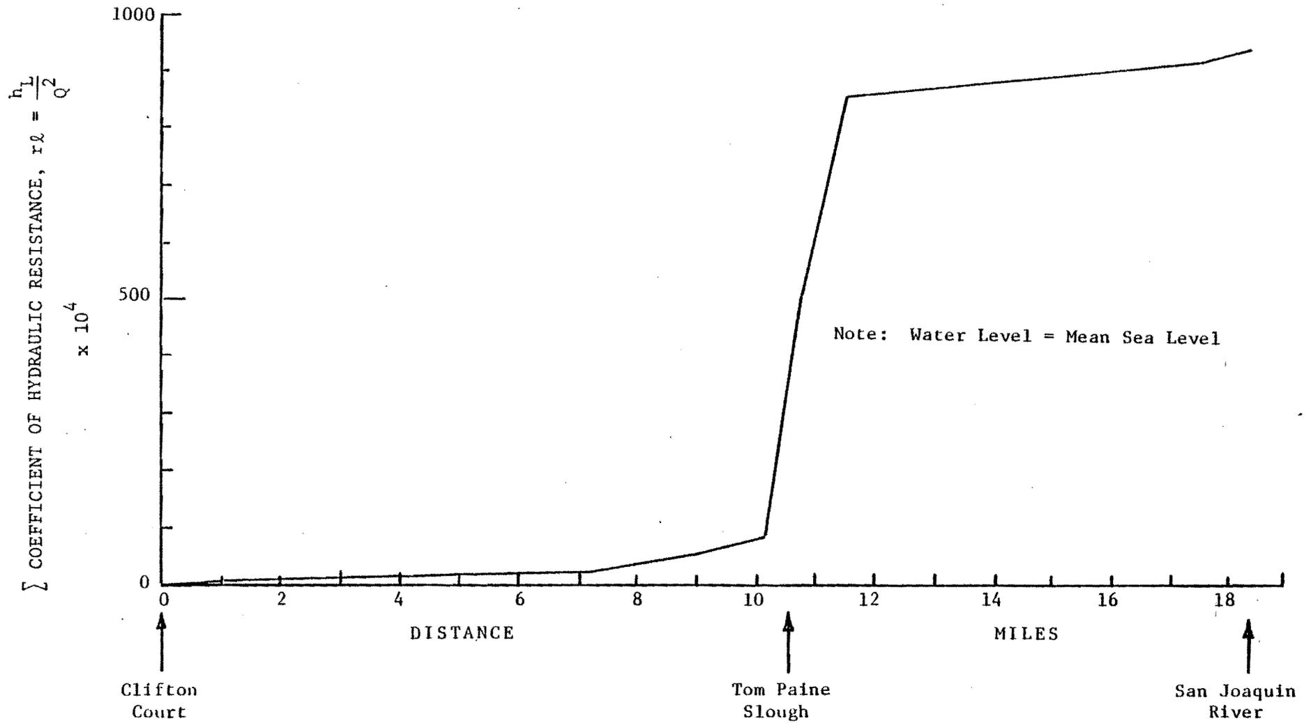
Figure VII-3 CUMULATIVE HYDRAULIC RESISTANCE IN OLD RIVER, CLIFTON COURT TO SAN JOAQUIN RIVER
