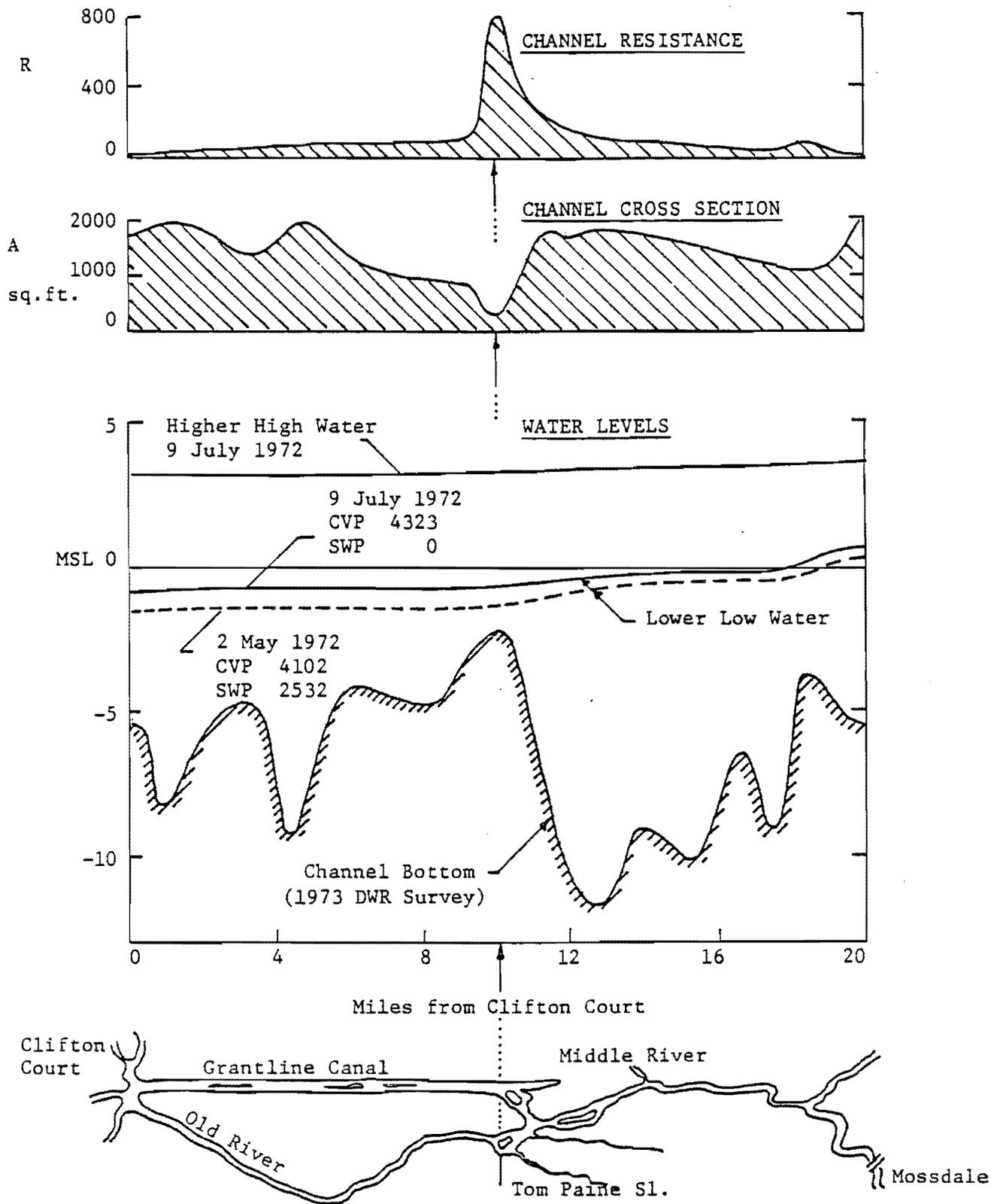
Figure VII-4 WATER LEVELS AND CHANNEL CHARACTERISTICS
