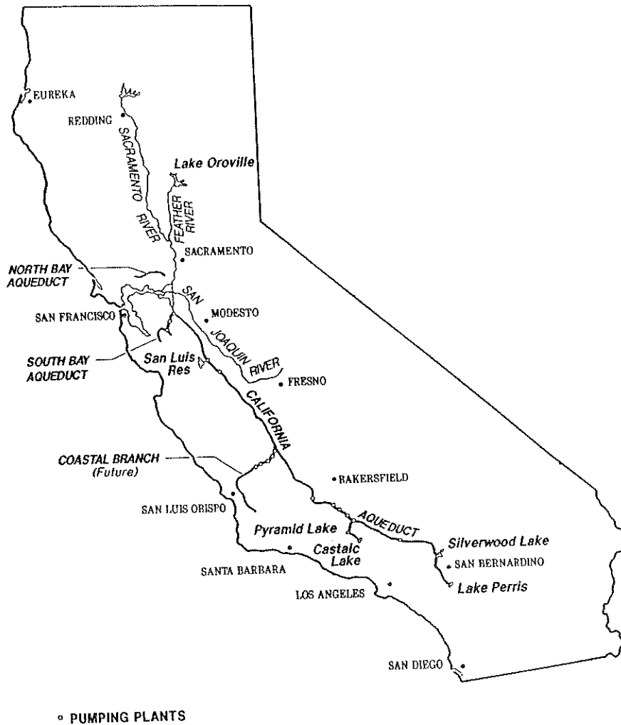
FIGURE 1. Major features of the California State Water Project.
