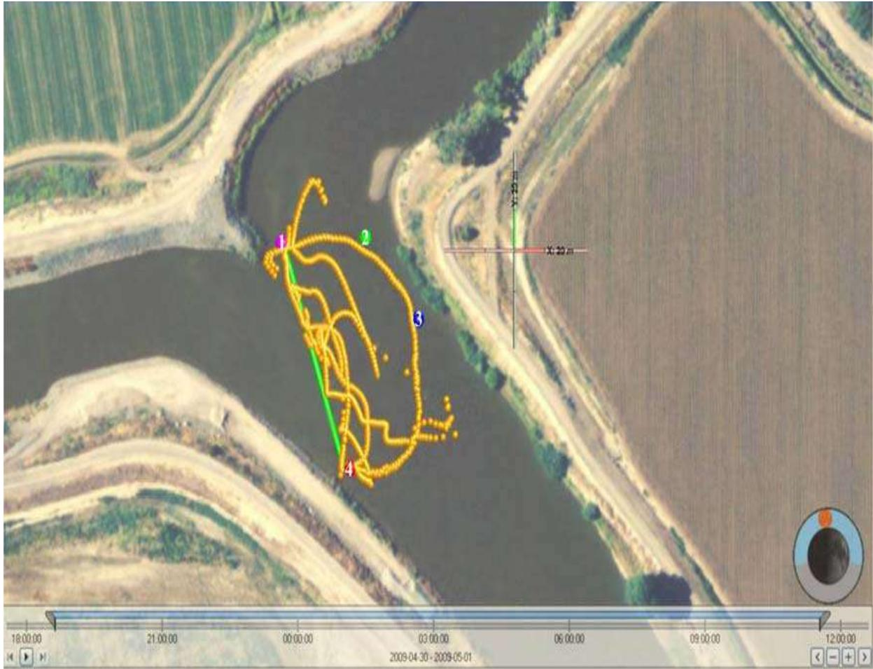
**Figure 8-3.** Acoustic tag tracking results for a juvenile Chinook salmon (yellow track) that was preyed upon in the vicinity of the non-physical barrier (green line) at the Head of Old River (Source Bowen *et al.* 2009).
