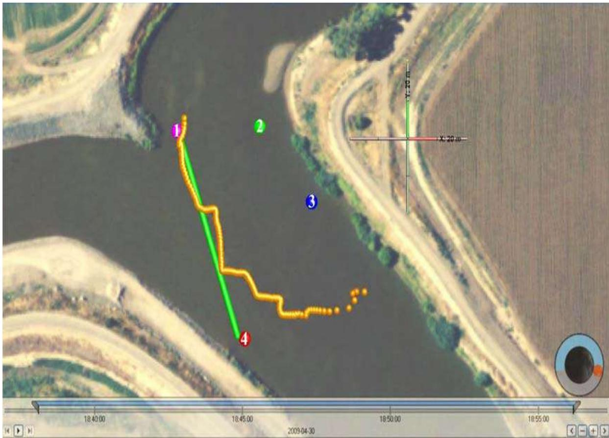
**Figure 8-2.** Acoustic tag tracking results for a juvenile Chinook salmon (yellow track) that was effectively guided downstream by the non-physical barrier (green line) at the Head of Old River (Source Bowen *et al.* 2009).
