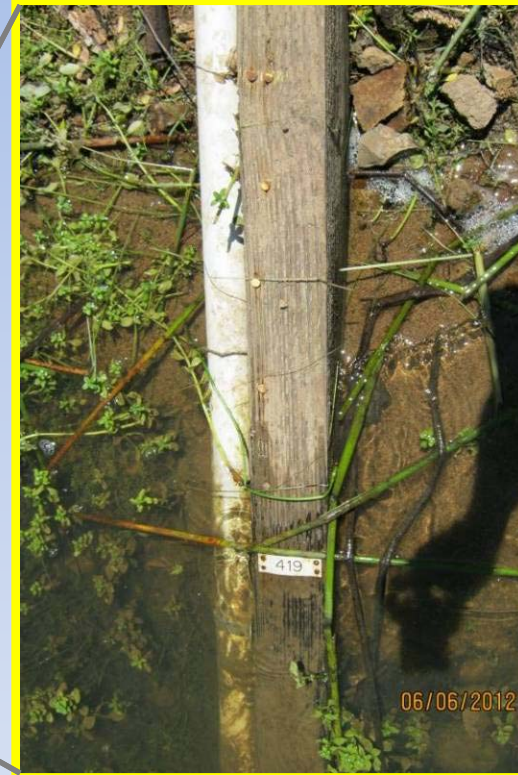
Detail Sloped Staff Gauge
