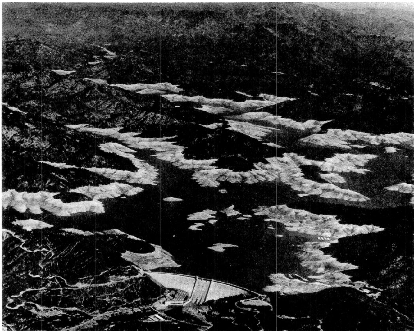
2. Low point for California's largest. Lake Shasta, formed at the junction of the McCloud, Pit, and Sacramento Rivers, is the primary facility of the federal Central Valley Project. This aerial photograph was taken on September 30, 1977, when the storage was 780 cubic hectometres (631,000 acre-feet), or only 20 percent of capacity. The low point was reached on September 14, 1977, with only 690 cubic hectometres (563,000 acre-feet).
