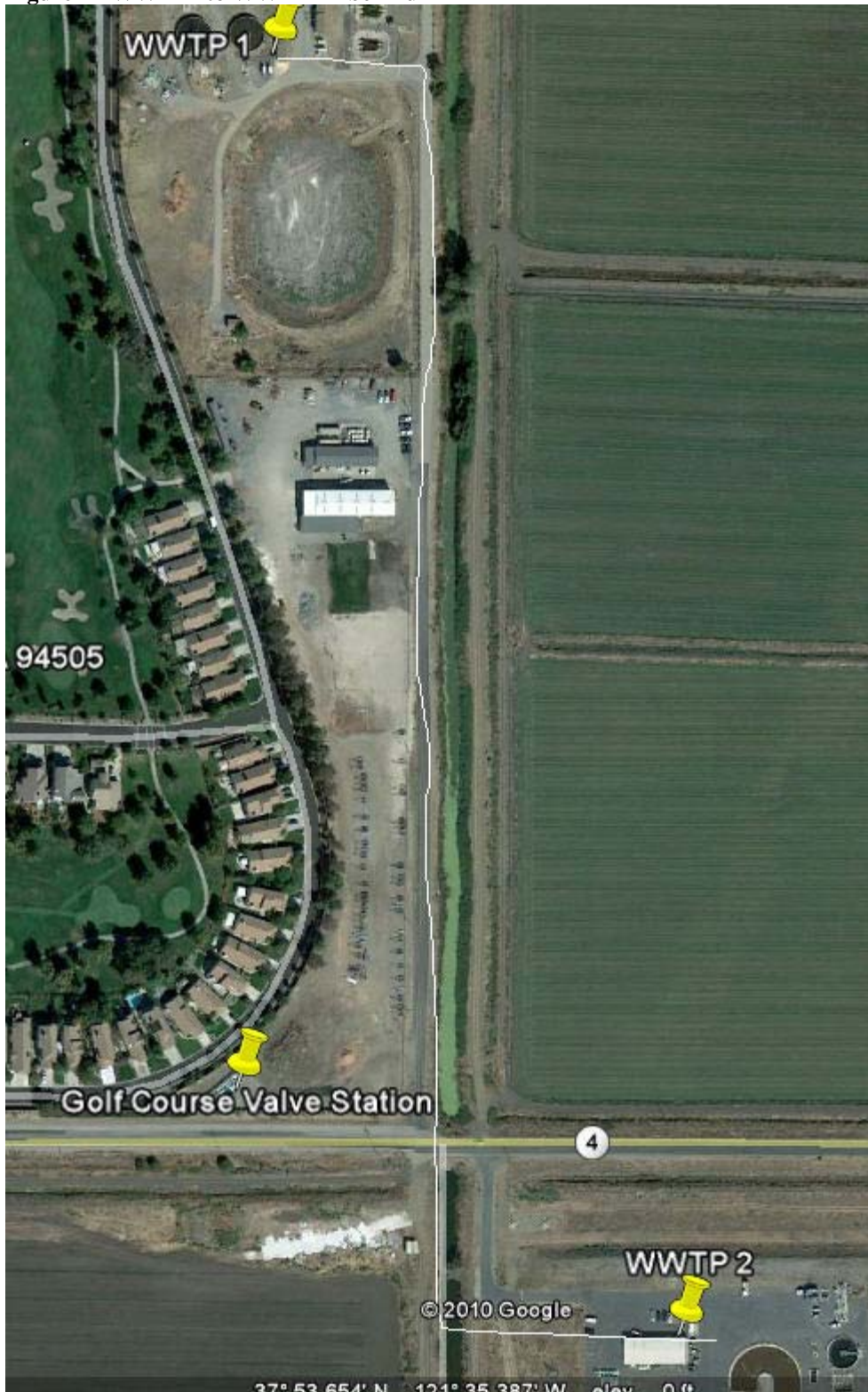
Figure 2 - WWTP1 to WWTP2 Fiber Run
