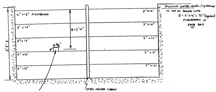
ORIFICE NOTCH MUST BE SIZED 4" x 4-3/8" with two 2"x 12" BOARDS BELOW AND TWO 2" x 12" BOARDS ABOVE BOARD WITH NOTCH
