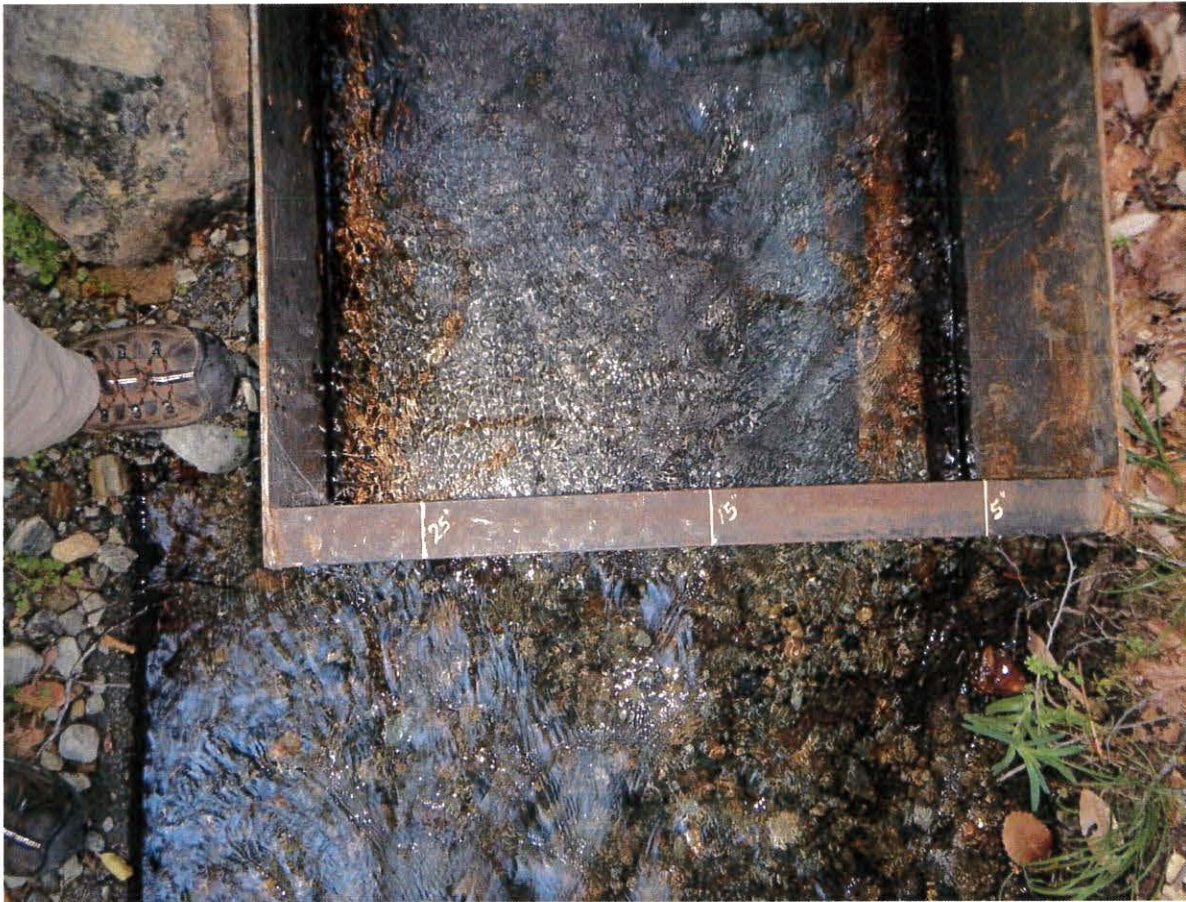
Photograph 13. Markings on metal bar indicate measurement locations.
