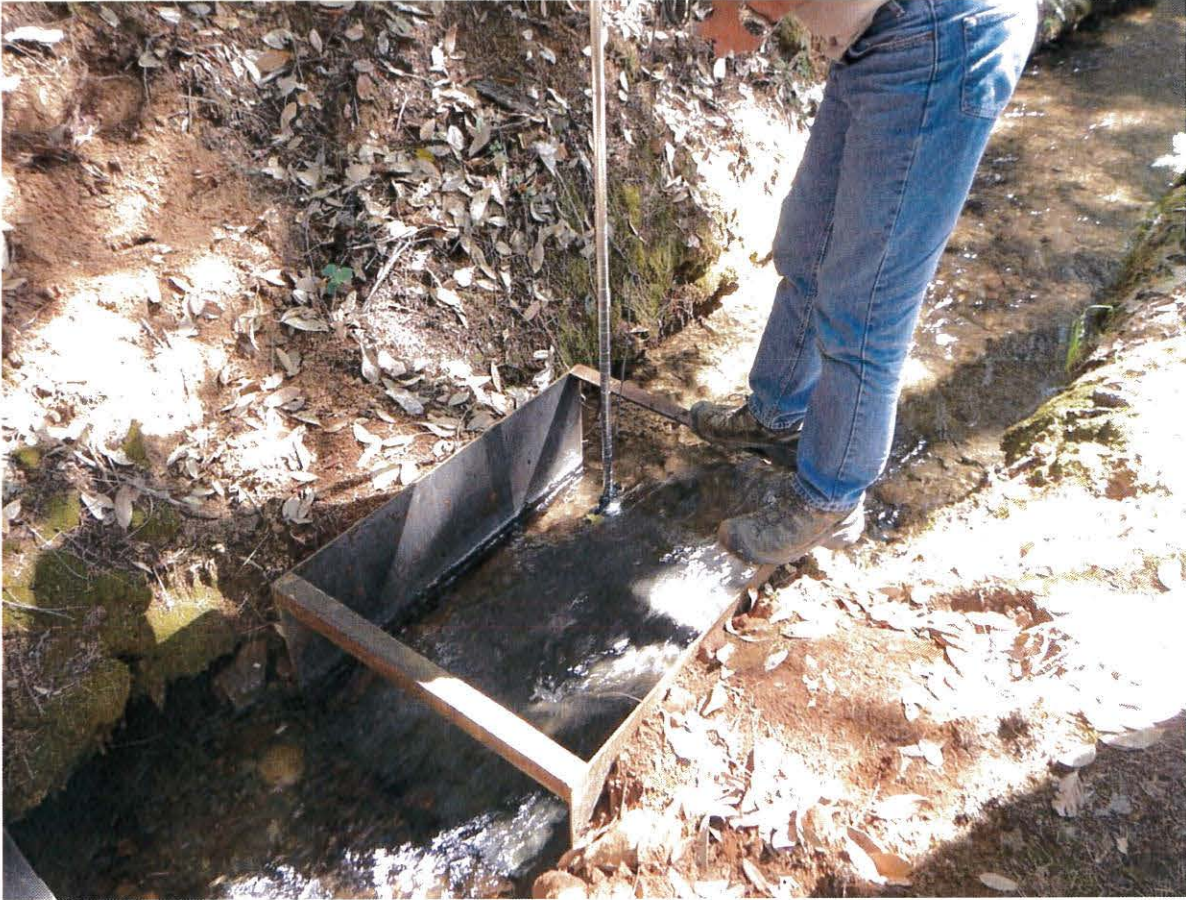
Photograph 15. Measurement conducted using Swiffer meter.
