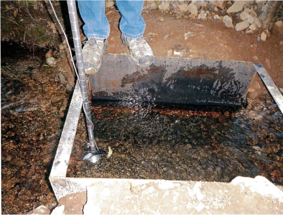
Photograph 14. Measurement conducted using Swoffer meter.
