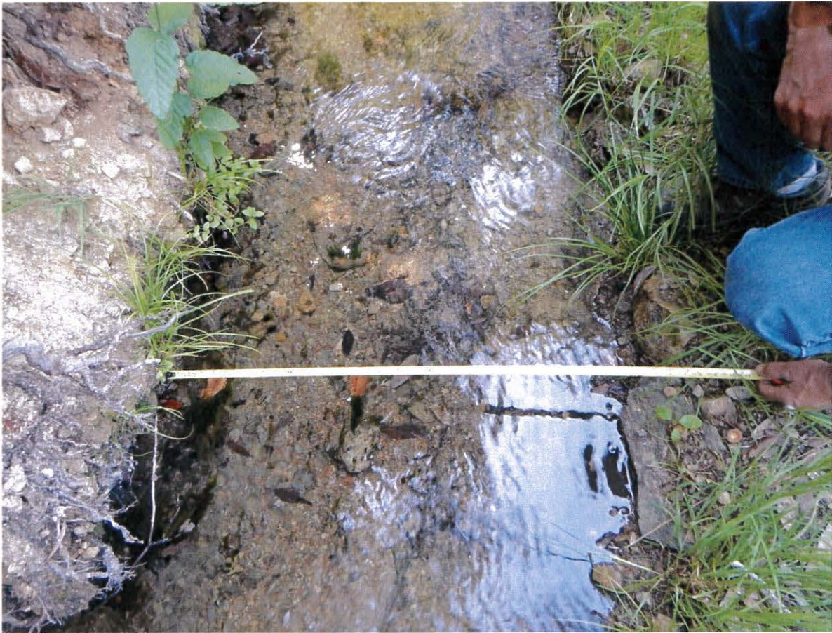
Photograph 11. Narrow location in canal, top width about 3.3 feet
