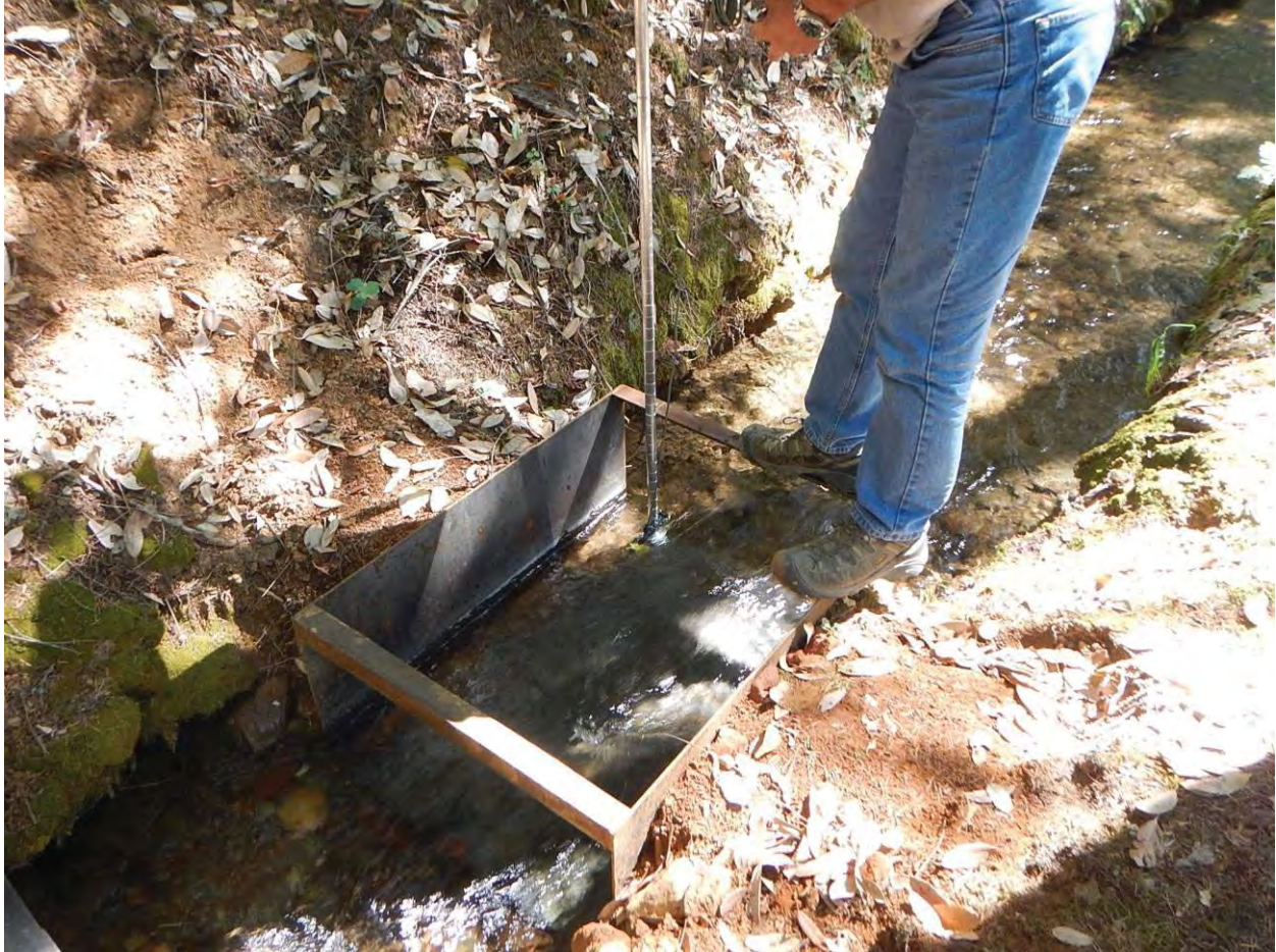
Photograph 15. Measurement conducted using Swiffer meter.
