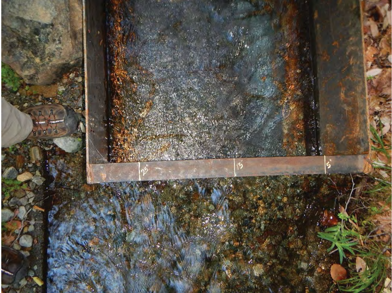
Photograph 13. Markings on metal bar indicate measurement locations.
