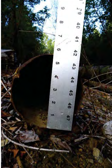
Photograph 3. Pipe adjacent to 14" Pipe. End of pipe was crimped making estimation of Interior diameter imprecise.
