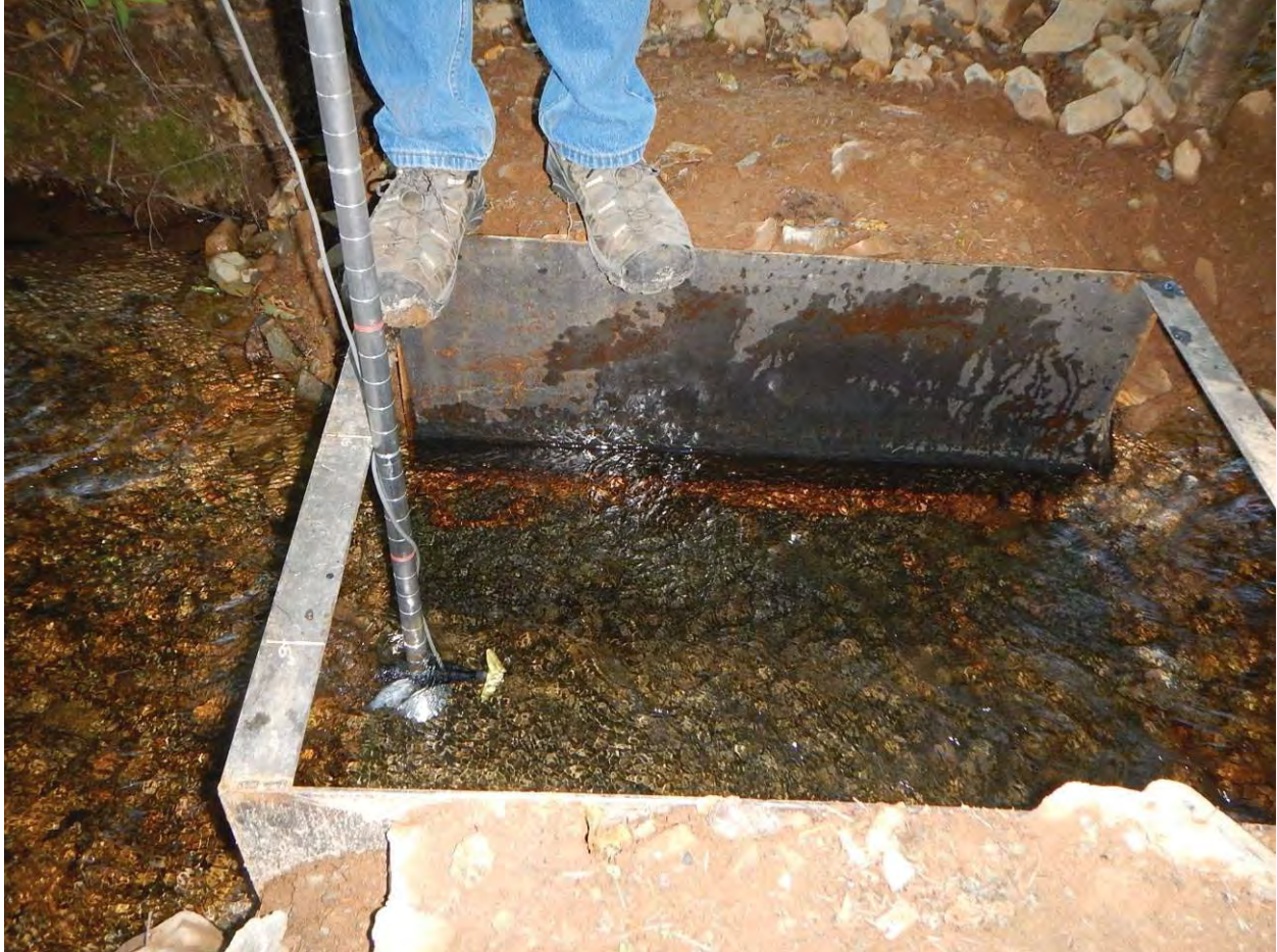
Photograph 14. Measurement conducted using Swiffer meter.
