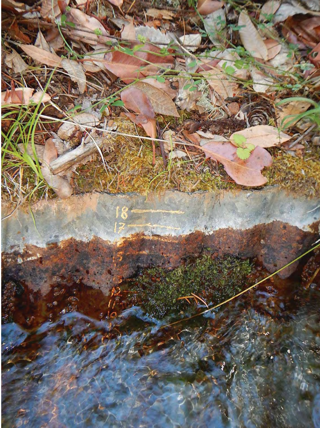
Photograph 8. Stanshaw Gage developed by Douglas Cole.
