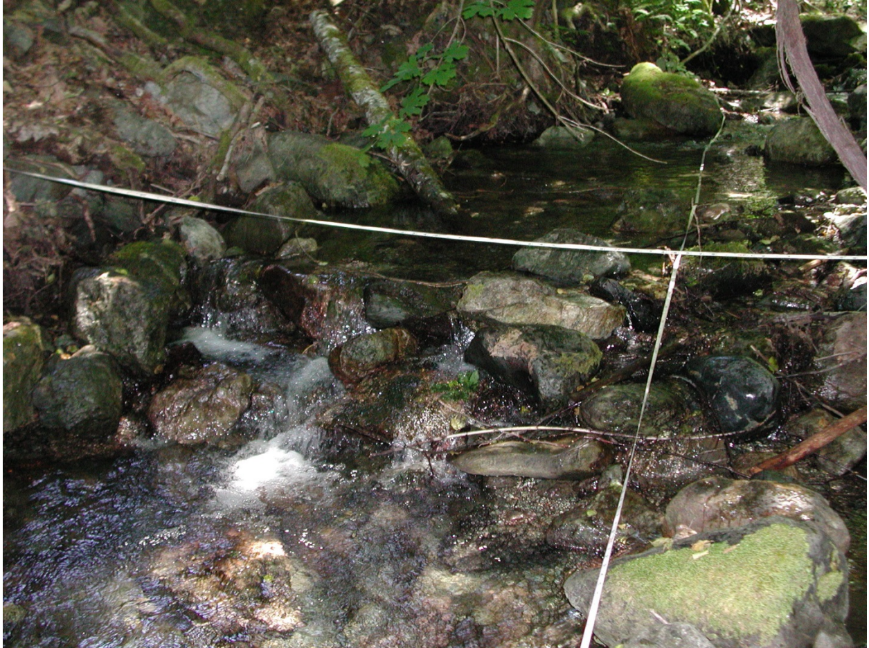
Figure 2 A cross section used in the hydraulic analysis in Stanshaw Creek (July 6, 2001).
