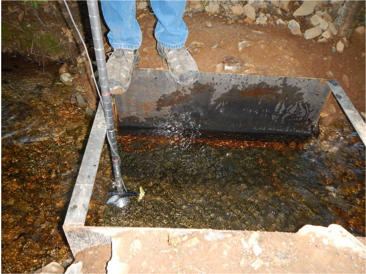
Photograph 14. Measurement conducted using Swiffer meter.
