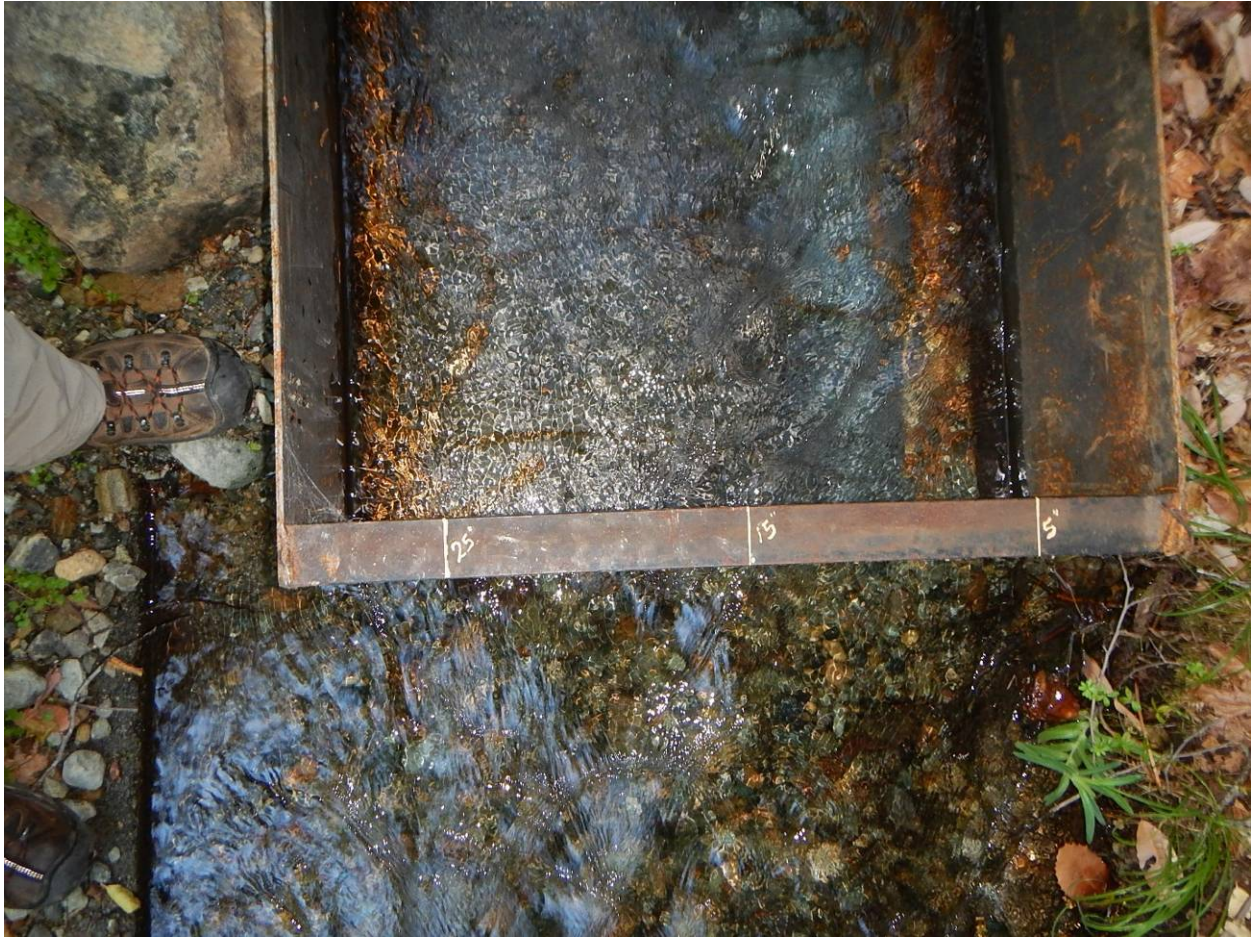
Photograph 13. Markings on metal bar indicate measurement locations.
