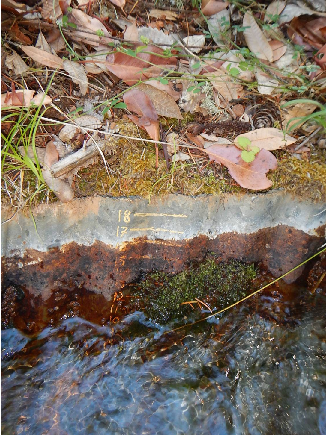
Photograph 8. Stanshaw Gage developed by Douglas Cole.
