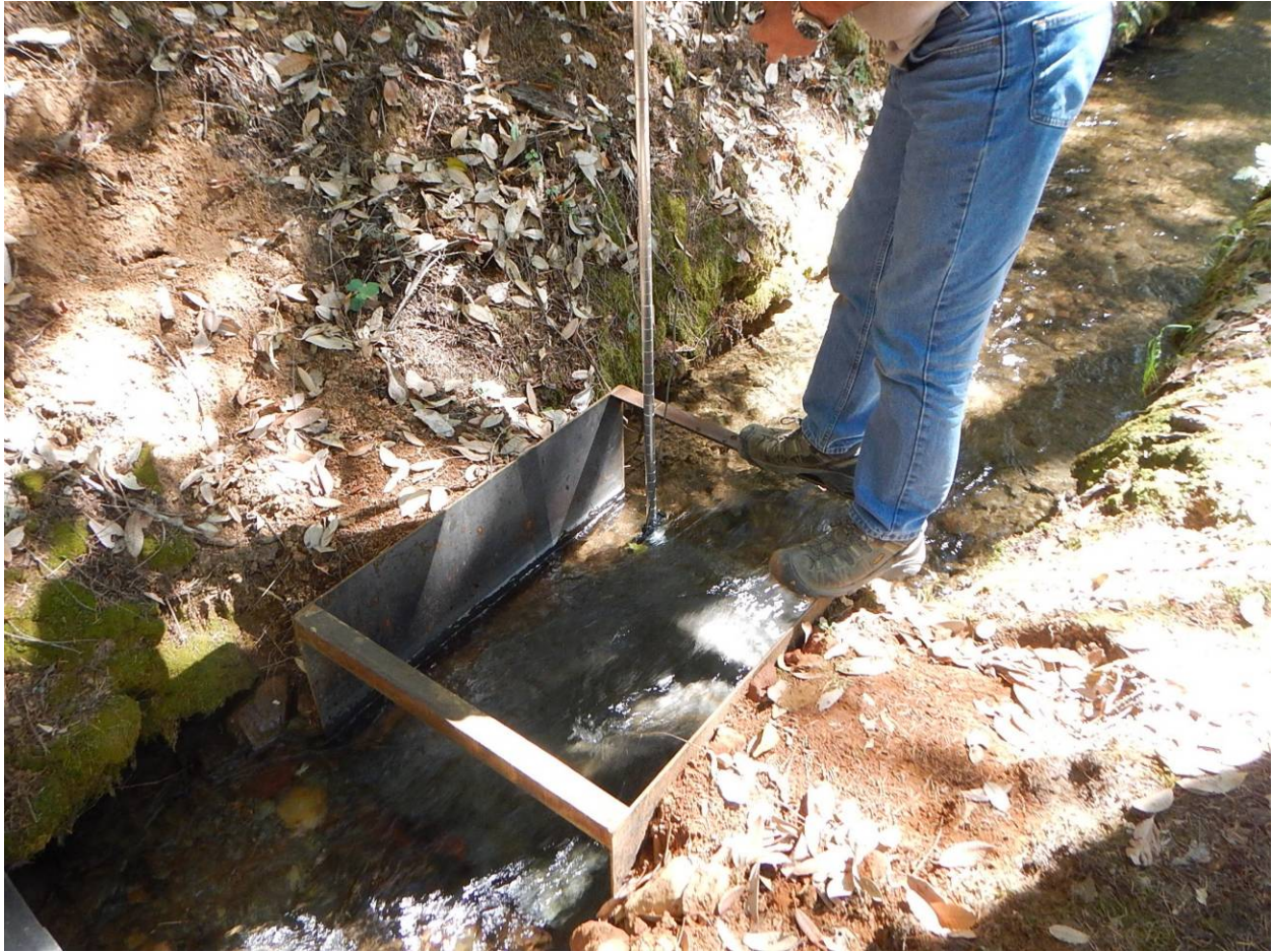
Photograph 15. Measurement conducted using Swiffer meter.
