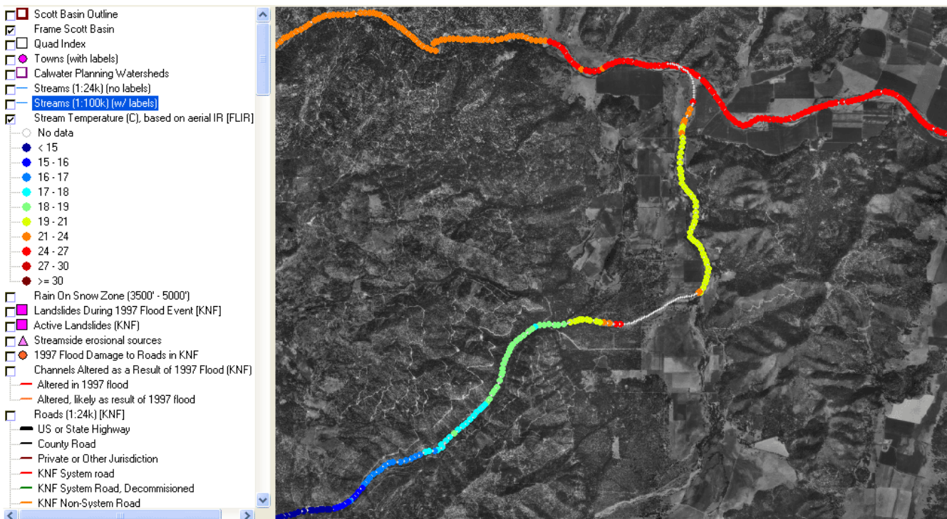
Figure 32. This map shows summary data of Scott River Thermal Infrared Radar (TIR) surveys for Shackleford Creek. Note that water temperature warms in a downstream direction as flow is depleted. Reaches with no temperature coded color are dry. Data from Watershed Sciences (2003).
