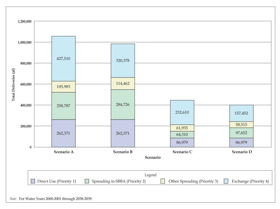
Figure 5.5-3. Projected Cumulative Total Initial Delivery of Captured SAR Water by Priority
