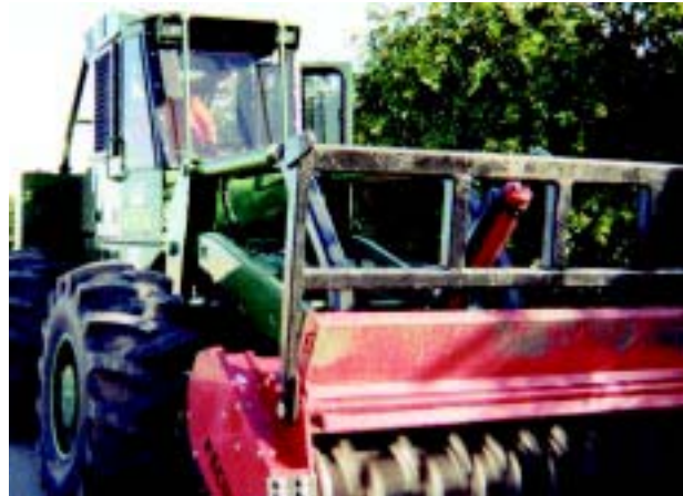
Arundo removal equipment used by Inland Empire West Resource Conservation District
