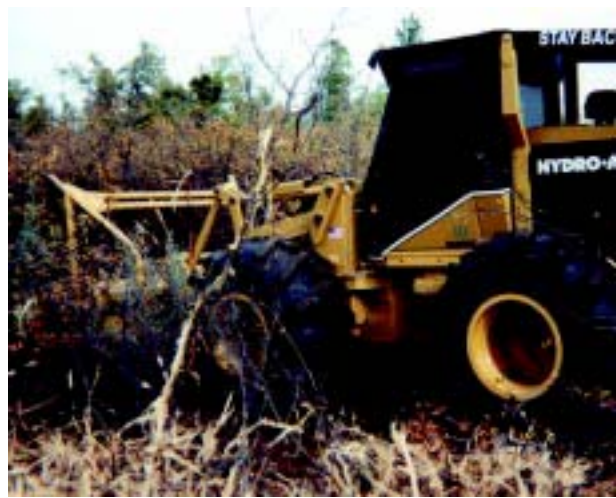
Hydro-Ax: Arundo removal equipment used by Inland Empire West Resource Conservation District (also used to clear fire breaks, as shown in this photo). Photo courtesy of Inland Empire West Resource Conservation District
