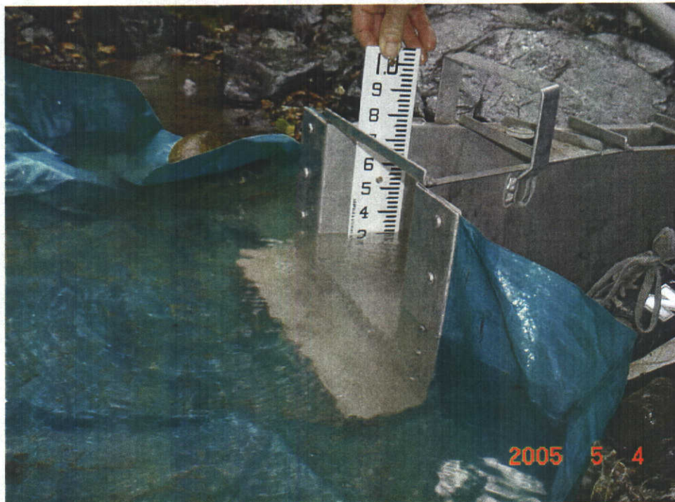
The depth of flow in the 3-inch Montana flume was 0.31 ft. This corresponds to about 0.16 cfs. It appeared that about 50% of the total streamflow was directed through the flume.
