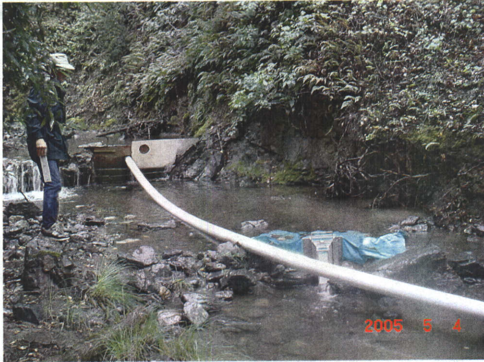
A flume was placed in the stream immediately below the POD to confirm compliance with the bypass. Due to the width of the stream, only a portion of the flow could be directed through the flume.
