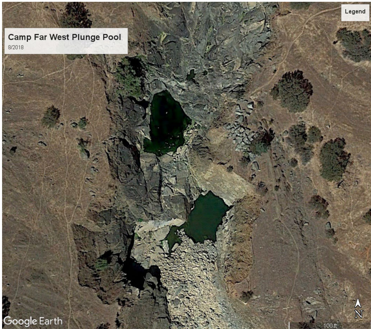
Figure A2. August 16, 2018 Google Earth aerial image of Camp Far West spillway plunge pool
