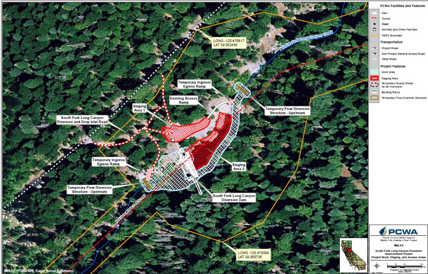
Figure A5. Aerial View of South Fork Long Canyon Diversion Improvement Project Staging Areas (PCWA 2023)
