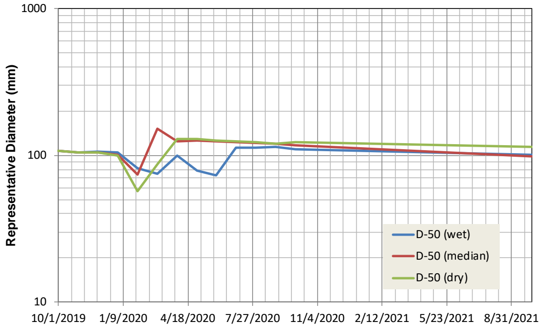
Figure 3.11-17. Simulated D50 (mm) from Iron Gate Dam to Bogus Creek during Successive Wet, Median, and Dry Water Years Following Reservoir Drawdown (Based on simulation results provided by USBR, March 2012).
