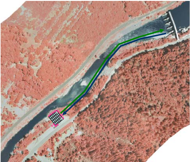
Figure 1c. Plan view of chiller location on Poe Reach; Pipe size = 4 ft; flow rate = 200 cfs
